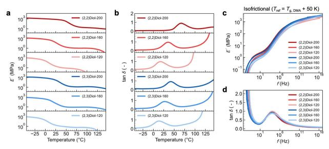
Fig. 3 Linear viscoelastic spectra of the copolymers. (a) Storage modulus E' at f=1.0 Hz as a function of temperature. (b) Loss tangent tan  $\delta$  as a function of temperature. (c) Isofrictional master curves of E' as a function of frequency f constructed at  $T_{\text{ref}} = T_{\text{g,DMA}} + 50$  K. (d) Loss tangent tan  $\delta$  as a function of f.
