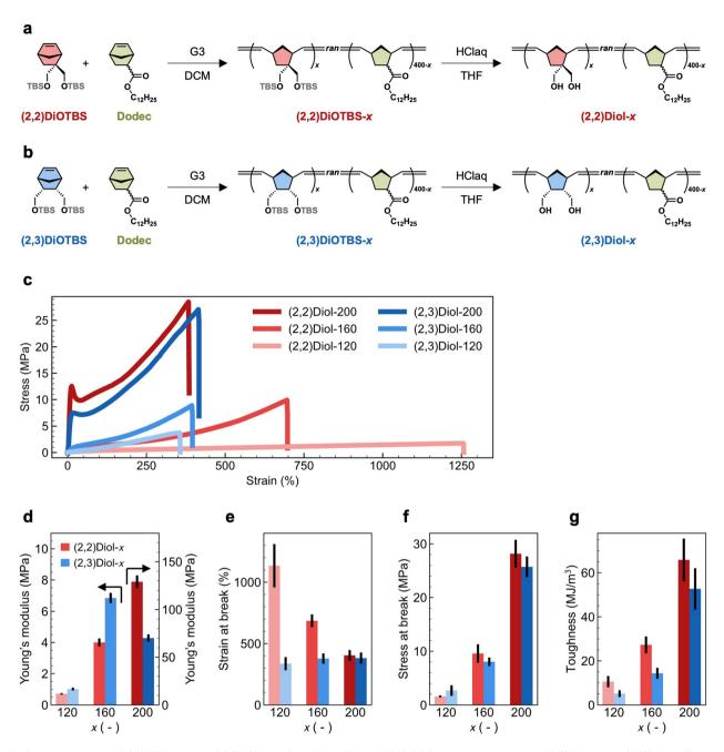
Fig. 1 Synthetic route of (a) (2,2)Diol-x and (b) (2,3)Diol-x (x = 120, 160, and 200). (c) Stress-strain curves of (2,2)Diol-x and (2,3)Diol-x. The tensile properties of (d) Young's modulus, (e) stress at break, (f) strain at break, and (g) toughness. Vertical black lines represent error bars indicating the standard deviation
