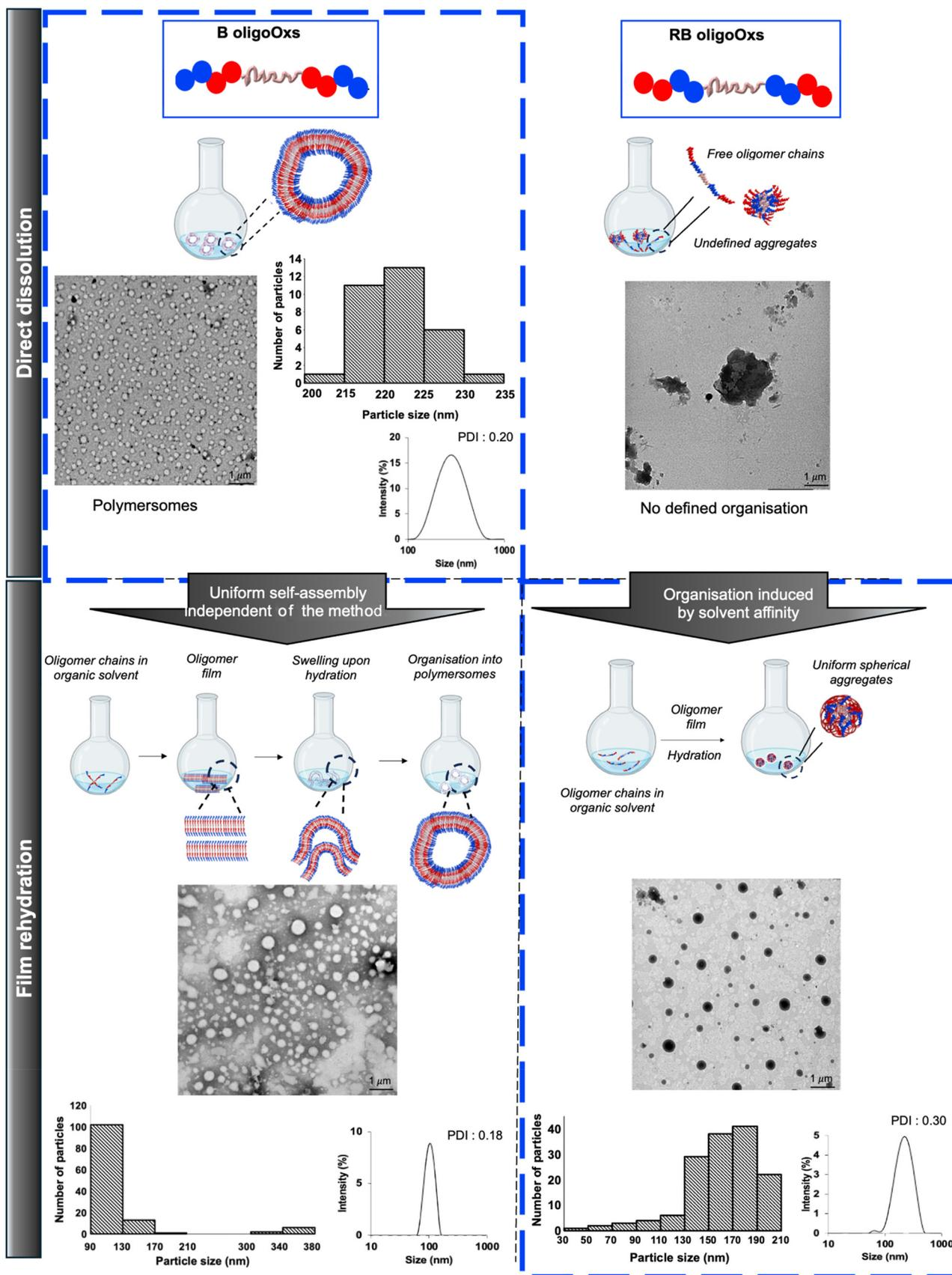
Fig. 4 Effect of oligoOx architectures B2 and RB2 and the preparation method on the self-assembly at 25 °C. Scale bar: 1  $\mu\text{m}$ . The contrast differences are assigned to the preference of the contrasting agent towards the imaging of hydrophilic compounds.
