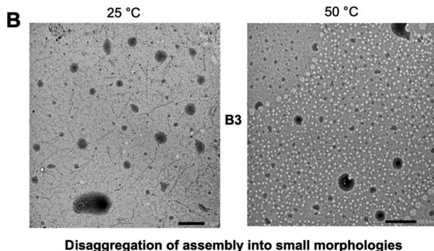
**Fig. 5** (A) Thermal transition temperature of block oligoOxs vs. pure PMeOx and PBuOx; (B) The temperature effect on the disaggregation of self-assembled B3 oligomers into smaller nano-objects. All measurements were recorded for a concentration of 1 mg mL<sup>-1</sup> in PBS. Scale bar: 1 μm.
