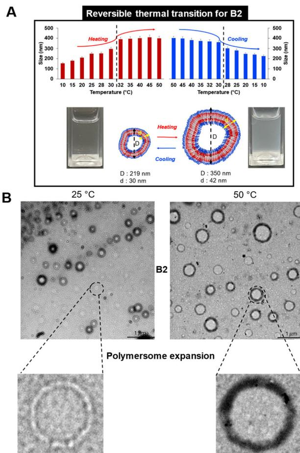
**Fig. 6** (A) Reversible polymersome shape transition for B2 evaluated by DLS and (B) TEM. All measurements were recorded for a concentration of 1 mg mL<sup>-1</sup> in PBS. Scale bar: 1 μm.
