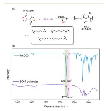
**Scheme 3** (a) Synthesis of cross-linked polyesters using bisDOX and diols. (b) FT-IR spectra of bisDOX showing its characteristic carbonyl stretching at 1790  $\,\mathrm{cm^{-1}}$  and BD-4 showing the appearance of a new C=O stretching peak at 1733  $\,\mathrm{cm^{-1}}$ .
