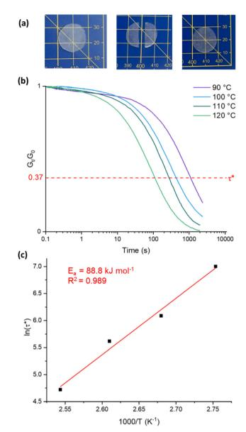
Fig. 2 (a) Pictures showing BD-10 before and after reprocessing by hot-pressing (b) stress-relaxation analysis for BD-10 indicating the characteristic relaxation time,  $\tau^*$ , when the relaxation modulus reaches 37% of its original value. (c) Arrhenius plot relating  $\tau^*$  to the inverse of temperature for BD-10.
