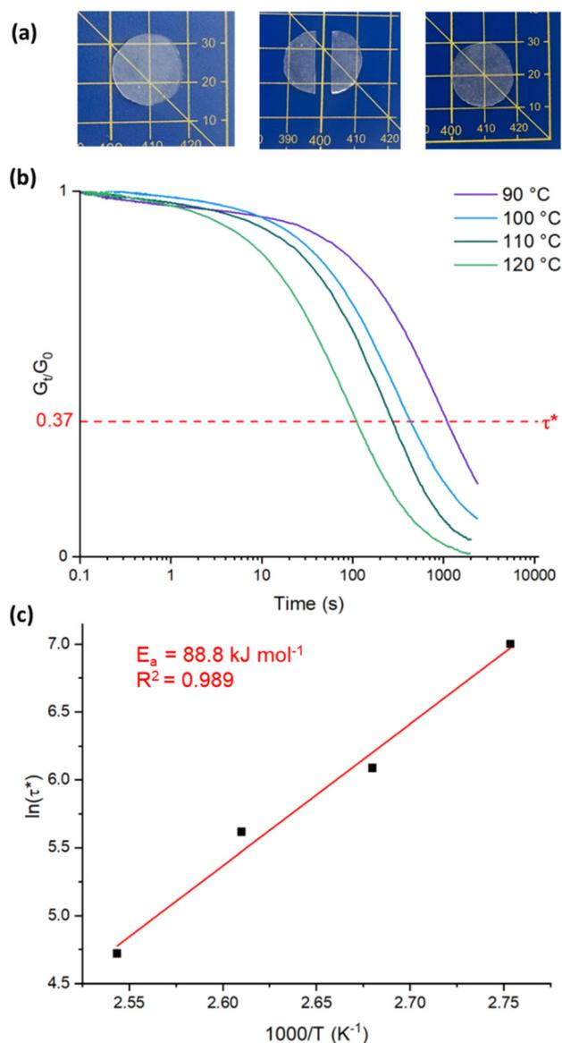
**Fig. 2** (a) Pictures showing **BD-10** before and after reprocessing by hot-pressing (b) stress-relaxation analysis for **BD-10** indicating the characteristic relaxation time,  $\tau^*$ , when the relaxation modulus reaches 37% of its original value. (c) Arrhenius plot relating  $\tau^*$  to the inverse of temperature for **BD-10**.
