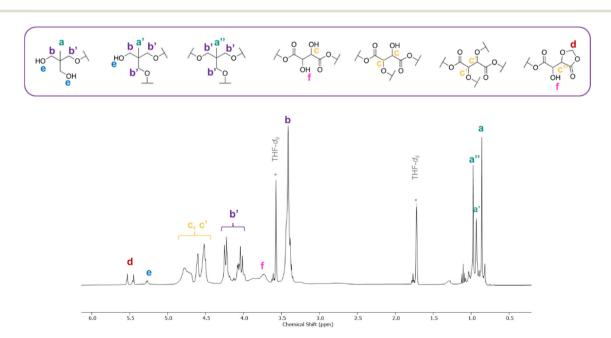
Fig. 1 <sup>1</sup>H NMR spectrum (THF-d<sub>8</sub>, 298 K, 500 MHz) of branched bisDOX and TME co-polymer showing possible different structural units.
