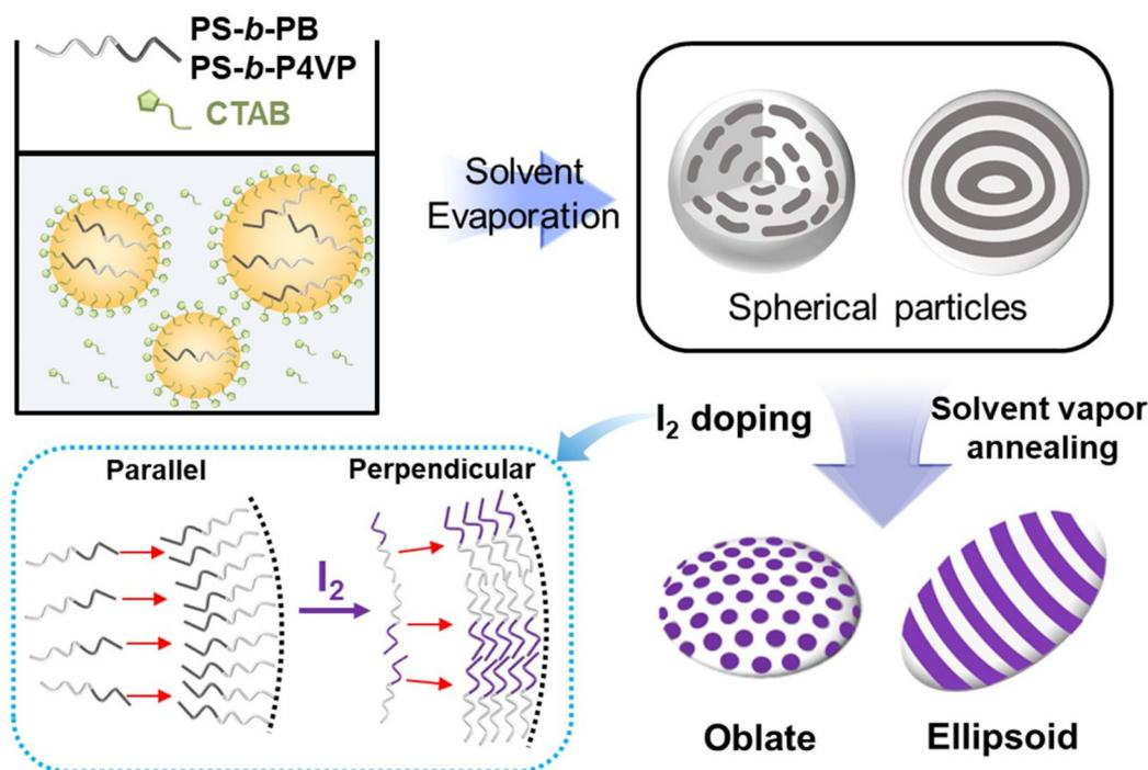
**Scheme 1** Experimental system showing the generation of spherical BCP particles *via* emulsion-solvent evaporation, followed by  $\text{I}_2$  doping to transform spherical BCP particles into oblates and ellipsoids.
