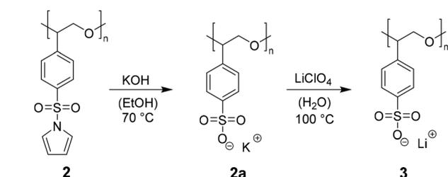
**Scheme 2** Synthesis protocol for the deprotection of **2** using a two-step approach; step 1: addition of KOH (10 eq. per monomer unit) in EtOH, 70 °C, reflux for 3 d to receive **2a**; step 2: salt metathesis using LiClO<sub>4</sub> (10 eq. per monomer unit) in H<sub>2</sub>O at 100 °C for 5 days.
