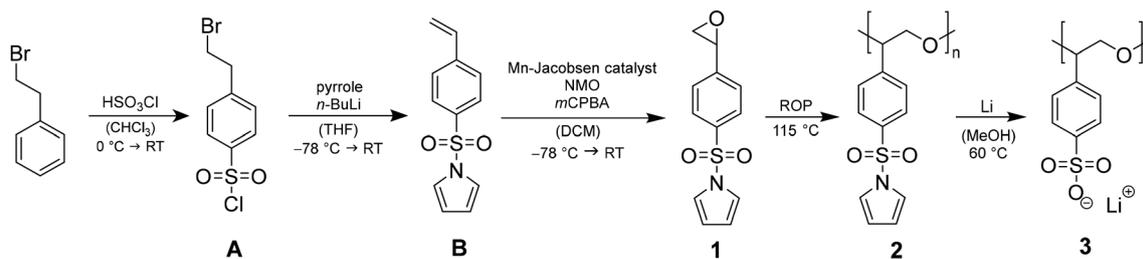
**Scheme 1** Three-step monomer synthesis including 1-((4-(oxiran-2-yl)phenyl)sulfonyl)-1H-pyrrole (**1**), catalytically supported anionic ROP of **1** to poly(1-((4-(oxiran-2-yl)phenyl)sulfonyl)-1H-pyrrole) (**2**) and cleavage of sulfonamide to obtain the final homopolymer poly(lithium 4-oxiran-2-yl)benzene sulfonate (**3**).
