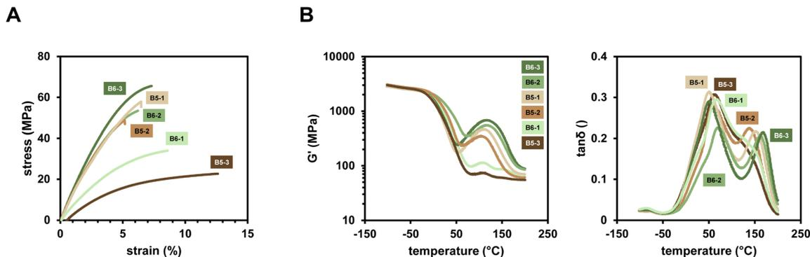
Fig. 7 (A) Stress/strain diagram derived from tensile tests of polymer samples using Mix-3 containing 0.2 mol% Cu(acac)<sub>2</sub> and 3.5 mol% diborane. (B) DMTA measurements depicting the storage modulus  $G'$  and the loss factor  $\tan(\delta)$  as a function of temperature (−100–200 °C). Samples were prepared from Mix-3 containing 0.2 mol% Cu(acac)<sub>2</sub> and 3.5 mol% diborane.
