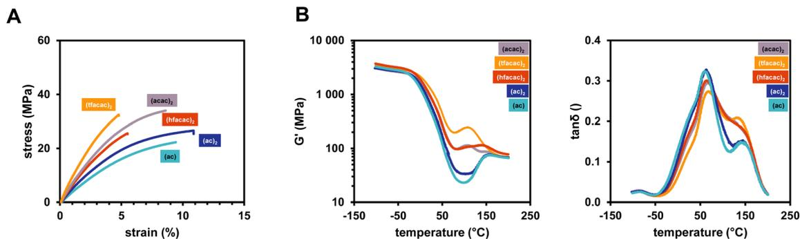
**Fig. 8** (A) Stress/strain diagram derived from tensile tests of polymer samples using Mix-3 containing 0.2 mol% copper salt and 3.5 mol% B6-1. (B) DMTA measurements depicting the storage modulus  $G'$  and the loss factor  $\tan(\delta)$  as a function of temperature ( $-100$ – $200$  °C). Samples were prepared from Mix-3 containing 0.2 mol% copper salt and 3.5 mol% B6-1.
