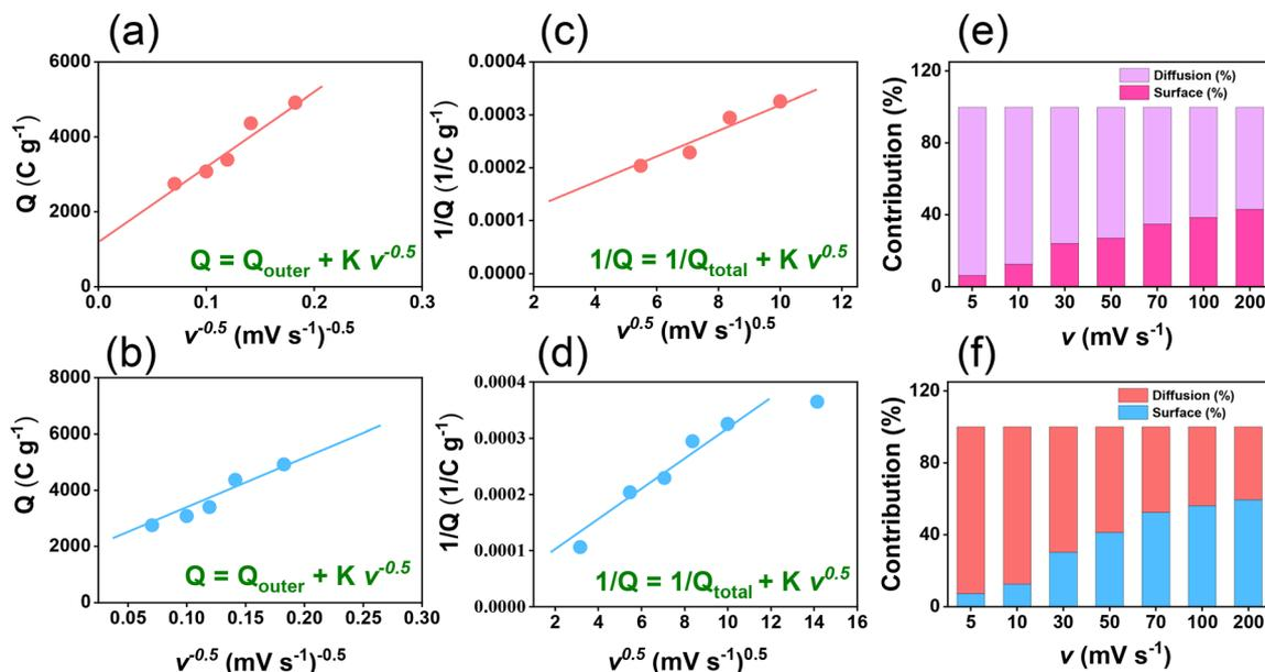
Fig. 5 (a and b) Relationship between  $Q$  ( $\text{C g}^{-1}$ ) and  $v^{-0.5}$  ( $\text{mV s}^{-1}$ ) $^{-0.5}$ , (c and d)  $1/Q$  vs.  $v^{0.5}$  ( $\text{mV s}^{-1}$ ) $^{0.5}$ , and (e and f) percentage of surface contribution and diffusion contribution for (a, c and e) TBN-Diyne CMP and (b, d and f) TPE-Diyne CMP electrodes.
