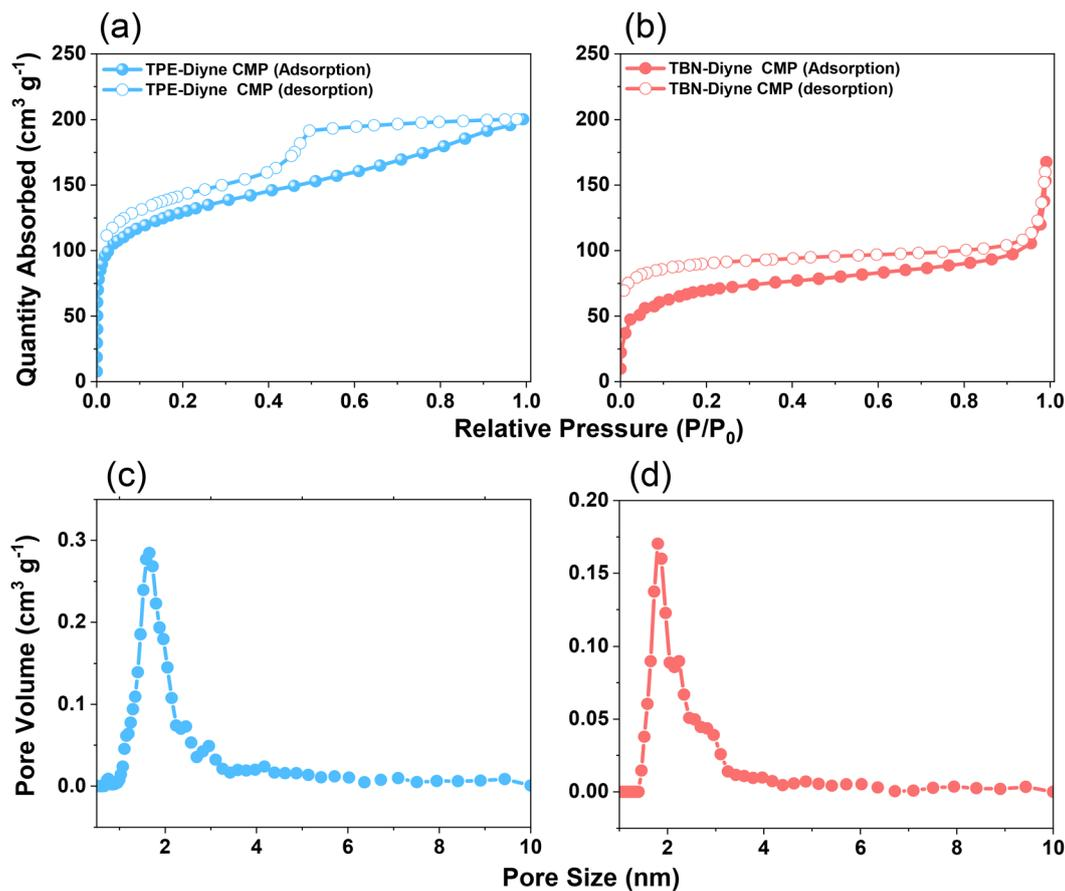
Fig. 3 (a and b)  $N_2$  sorption isotherms and (c and d) PSD profiles of the TPE-Diyne CMP (a and c) and TBN-Diyne CMP (b and d).
