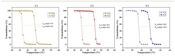
Fig. 2 Transmittance plotted as a function of solution temperature for the  $T_{cp}$  determination of polymers C1, C2 and C3 (from left to right) in both D<sub>2</sub>O and H<sub>2</sub>O.
