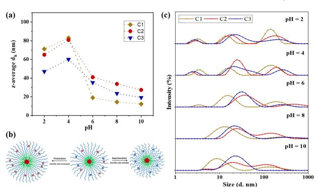
Fig. 5 (a) Changes in the z-average  $d_h$  against different pH values for C1, C2, and C3. (b) Schematic demonstrating the impact of protonation on the terpolymer (C3) and its sizes. (c) Particle size distribution by intensity under varying pH levels: 2, 4, 6, 8, and 10.
