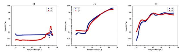
Fig. 8 Rheological measurements during a 1 °C min<sup>-1</sup> temperature scan from 20 to 65 °C under a constant shear strain of 1% ( $\gamma$ ) for C1–C3 dissolved in PBS at 20% w/w.
