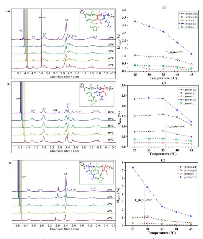
Fig. 3 Temperature-variation <sup>1</sup>H NMR spectra and corresponding proton integration ratios for a 10.0 mg mL<sup>-1</sup> sample of (a) C1, DMA<sub>32</sub>-b-MMA<sub>25</sub>b-NMEP<sub>20</sub> (b) C2, MMA<sub>22</sub>-b-DMA<sub>31</sub>-b-NMEP<sub>18</sub> and (c) C3, MMA<sub>21</sub>-b-NMEP<sub>18</sub>-b-DMA<sub>34</sub> in D<sub>2</sub>O to that of H<sub>2</sub>O (I/I<sub>H,O</sub>), plotted as a function of solution temperature.
