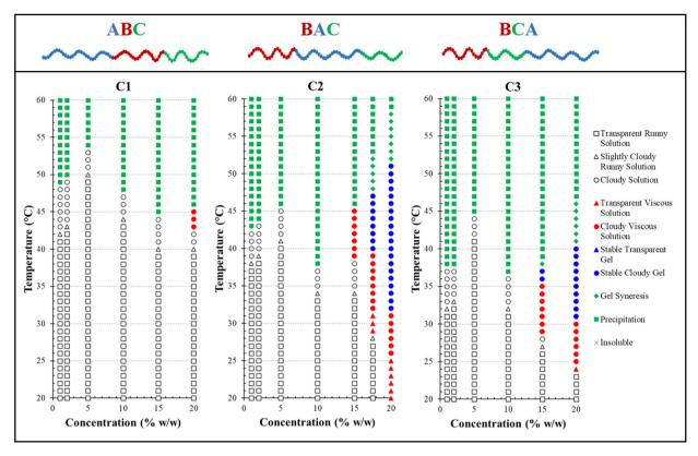
Fig. 7 Phase diagram of C1–C3, plotted using visual observation results for polymer solutions prepared in PBS (pH = 7.4) at concentrations of 1% w/w, 2% w/w, 5% w/w, 10% w/w, 15% w/w, and 20% w/w. Visual transition states are reported as: (a) runny solution in white, (b) viscous solution in red, (c) stable gel in blue, and (d) phase separation in green.
