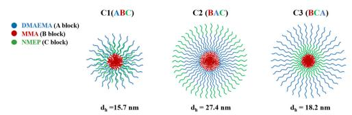
Fig. 4 Schematic representation of the proposed micelle configuration and the hydrodynamic diameters as measured by DLS for C1, C2, and C3.
