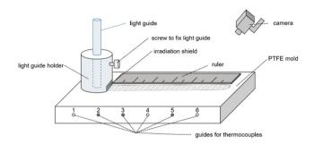
Fig. 3 Schematic illustration of the frontal polymerization setup A.
