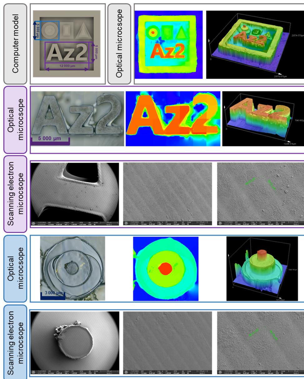
Fig. 11 Photographs of a print made from an **Az2** derivative-based resin obtained using an optical microscope and a scanning electron microscope.
