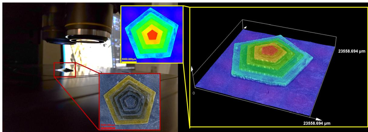
**Fig. 10** Images of the first 3D object obtained by 3D printing including a panoramic photo of the print, a panoramic photo showing the differences in the heights of individual layers and 3D visualization of the heights of individual parts of the print.
