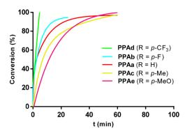
Fig. 5 Time-conversion plots for the polymerization of ring-substituted phenylacetylene derivatives. Reaction conditions: THF, 20 °C,  $[PA]_o = 0.25 \text{ M}$ ,  $[PA]_o/[Rh] = 100$ .
