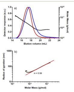
Fig. 3 (a) SEC chromatograms: light scattering detector response (90 degrees) (red) and differential refractometer response (blue), MM (molar mass) vs. elution volume plot for a PPAe sample prepared from PAe (R = p-OMe). (b) Log-log plot of the radius of gyration ( $r_0$ ) vs. MM.
