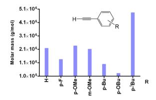
Fig. 2 Molar mass ( $M_w$ ) of the polymer samples obtained by polymerization of ring-substituted phenylacetylene derivatives catalyzed by [Rh (nbd){ $\kappa^2 P, N-Ph_2 P(CH_2)_3 NMe_2$ }][BF<sub>4</sub>].
