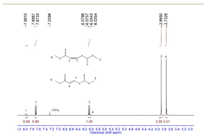
**Fig. 3** <sup>1</sup>H-NMR spectrum for the product **1** from COS, MP, and methanol.
