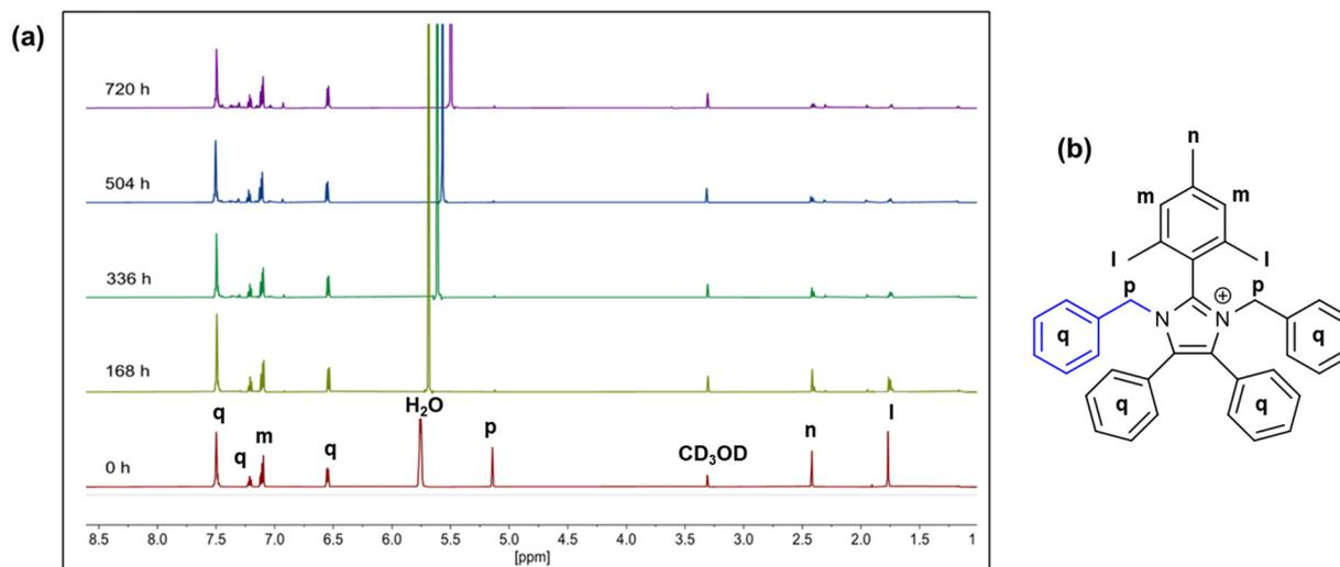
Fig. 3 (a) <sup>1</sup>H NMR of a representative compound **7d** in 3 M NaOD/CD<sub>3</sub>OD/D<sub>2</sub>O at 80 °C at various intervals over 720 h. (b) Proton labeling of compound **7d**.
