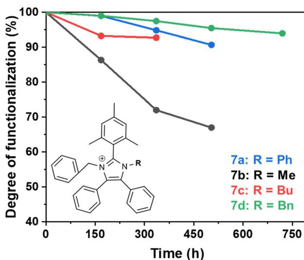
Fig. 4 The degree of functionalization remaining after the alkaline degradation test performed on synthesised molecules in 3 M NaOD/CD<sub>3</sub>OD/D<sub>2</sub>O at 80 °C at various intervals over 720 h.
