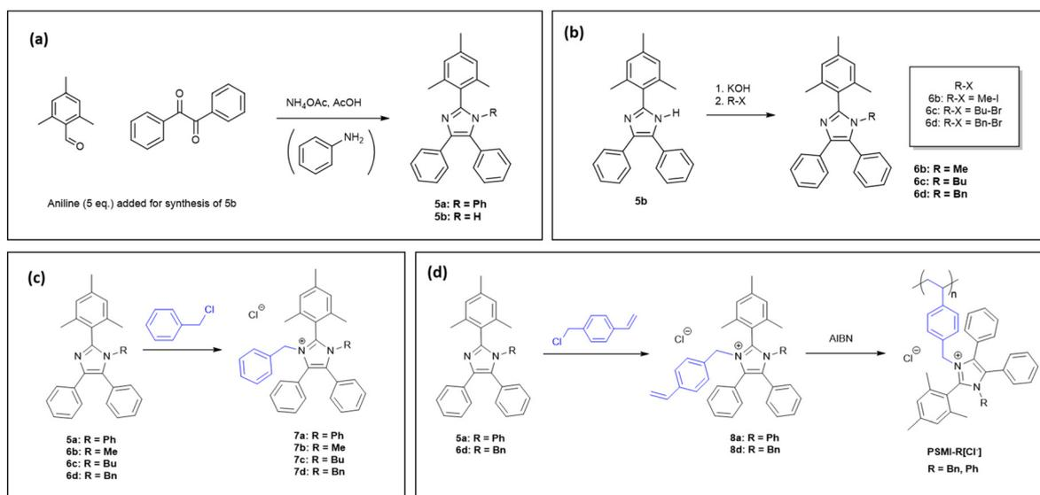
**Fig. 1** (a) Synthesis of imidazole monomer precursors (b) first *N*-functionalisation step (c) second *N*-functionalisation step for synthesis of imidazolium model compounds (d) second *N*-functionalisation for monomer synthesis followed by polymerisation.
