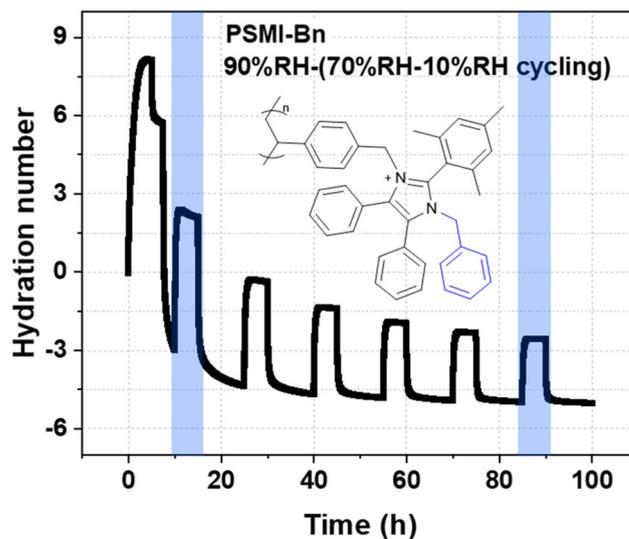
Fig. 7 DVS curve collected at 80 °C. The change in weight is monitored *via* the change in hydration number assuming a constant theoretical IEC of 1.7 mmol g<sup>-1</sup>. Initial 5 h of experiment at 85 %RH was conducted to condition the polymer and collect a maximum accessible water uptake and hydration number value.
