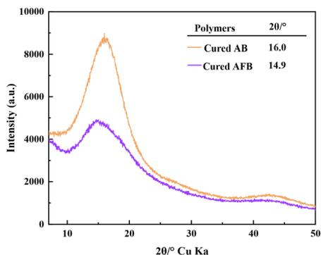
**Fig. 6** X-ray diffraction patterns of cured AB and cured AFB.
