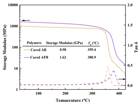
Fig. 4 DMA curves of cured **AB** and cured **AFB** at a heating rate of 5 °C min<sup>-1</sup> in N<sub>2</sub>.
