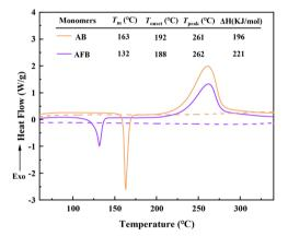
Fig. 1 DSC traces of AB and AFB at a heating rate of 10 °C min<sup>-1</sup>.
