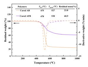
Fig. 3 TGA curves of AB and AFB at a heating rate of 10 °C min<sup>-1</sup> under N<sub>2</sub>.
