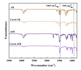
Fig. 2 FT-IR spectra of AB, AFB, cured AB and cured AFB.
