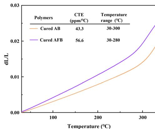
Fig. 5 CTE curves of cured **AB** and cured **AFB** at a heating rate of 5 °C min<sup>-1</sup> in N<sub>2</sub>.
