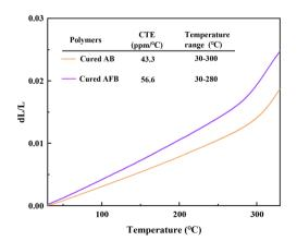
Fig. 5 CTE curves of cured AB and cured AFB at a heating rate of 5 °C
