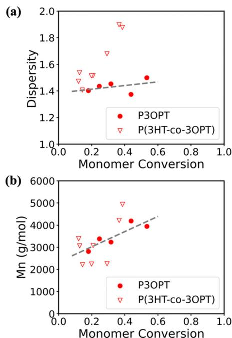
Fig. 6 (a) Dispersities of P3OPT and P(3HT-co-3OPT) vs. the monomer conversion and (b)  $M_n$  change of P3OPT and P(3HT-co-3OPT) vs. the monomer conversion. Here,  $M_n$  values were obtained from GPC measurements.
