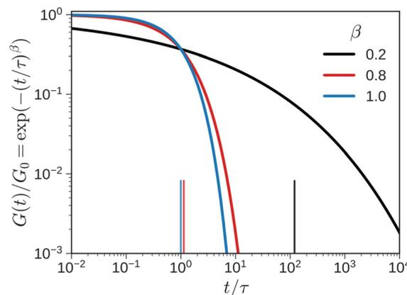
Fig. 17 The stretched exponential function for three different values of the stretching parameter.  $\beta = 1$  (blue line) corresponds to  $e^{-t/\tau}$ . The vertical lines on the horizontal axis mark the terminal relaxation time,  $\tau_{\text{term}}^{(1)}$ , for different  $\beta$ .
