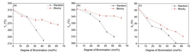
Fig. 8 The (a)  $T_{C_s}$  (b)  $T_{m_s}$  and (c)  $X_c$  as a function of degree of bromination for blocky (red, circles) and random (black, squares) BrPEKK. Dashed lines are to guide the eye.
