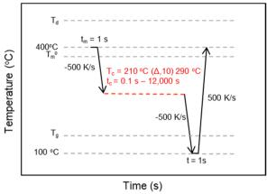
Fig. 2 The time-temperature profile for the Flash DSC interrupted isothermal crystallization (IIC) method used to determine the  $t_{1/2}$  of BrPEKK copolymers at a range of  $T_{\rm iso}$ .
