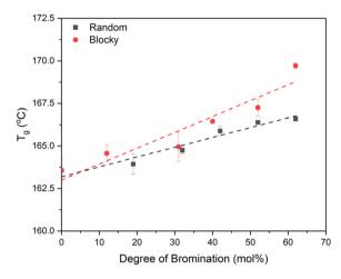
Fig. 9 Glass transition temperatures  $(T_q)$  of random (black squares) and blocky (red circles) amorphous BrPEKK determined from the midpoint of amorphous samples.
