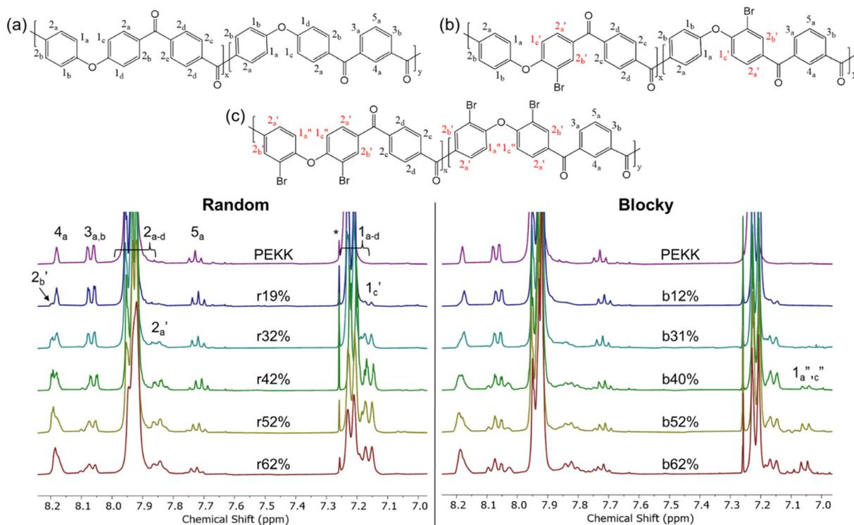
Fig. 5 <sup>1</sup>H NMR of random (left) and blocky (right) brominated PEKK up to 62 mol% bromination and the corresponding chemical structures of (a) pristine PEKK, (b) monosubstituted BrPEKK, and (c) disubstituted BrPEKK. Assignments are further verified by 2D NMR in the ESI.† Spectra are referenced to CDCl<sub>3</sub>. The asterisk (\*) refers to reference solvent resonance.
