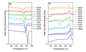
Fig. 7 Standard DSC scans of blocky (solid lines) and random (dashed lines) BrPEKK (a) first cool after removal of thermal history and (b) second heat. All DSC scans were performed at 10 °C min<sup>-1</sup> in a nitrogen atmosphere.
