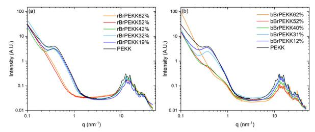
Fig. 11 Small, mid, and wide-angle X-ray scattering profiles of (a) random BrPEKK and (b) blocky BrPEKK. All samples were isothermally crystallized from the melt at 280 °C for 30 minutes in a nitrogen atmosphere.
