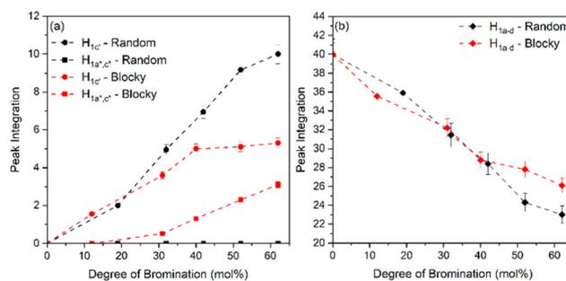
Fig. 6 Peak integration versus degree of bromination of (a) monosubstituted,  $H_{1c'}$  (circles), disubstituted,  $H_{1a'',c''}$  (squares) and (b) unsubstituted,  $H_{1a-d}$  (diamonds) random (black) and blocky (red) BrPEKK. The blocky microstructure shows an increase in disubstituted monomers due to the chemical confinement effect of gel state functionalization.
