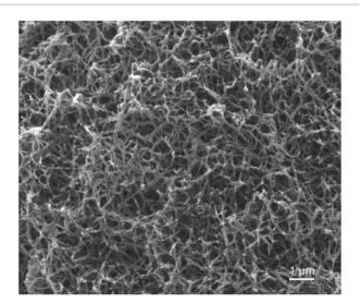
Fig. 3 SEM image of 15 wt% PEKK aerogel gelled from DPA.
