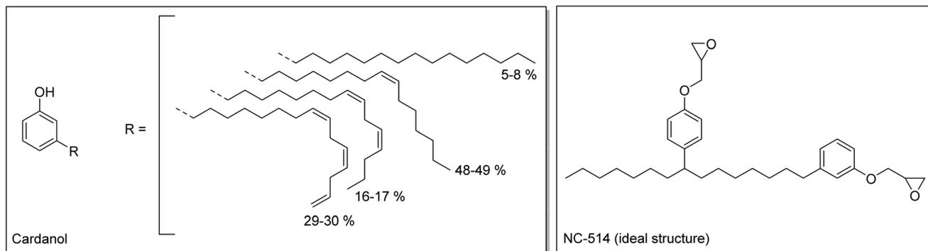
Scheme 3 Structures of cardanol<sup>42</sup> and of NC-514 (ideal structure expected).
