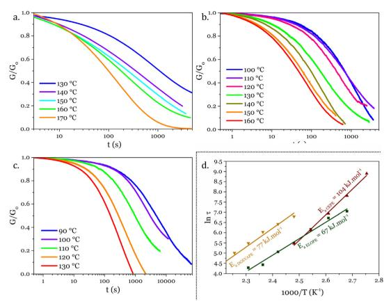
Fig. 5 Stress-relaxation experiments results on (a) DGEVAPE, (b) ELOPE and (c) CEPE. (d) Arrhenius diagram of the  $\tau$  determined from Kohlrausch–Williams–Watt fits for each material, and determination of the flow activation energies.
