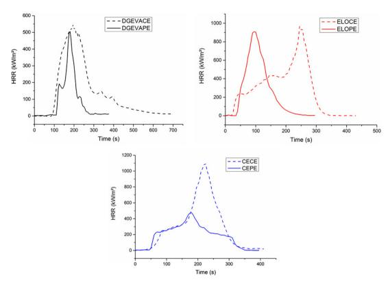
Fig. 8 Cone calorimeter curves of the phosphate ester vitrimers DGEVAPE, ELOPE, CEPE and their carboxylic ester counterparts DGEVACE, ELOCE, CECE
