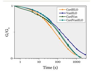
Fig. 10 Stress-relaxation experiments on epoxy mixtures vitrimers at 150  $^{\circ}\text{C}.$
