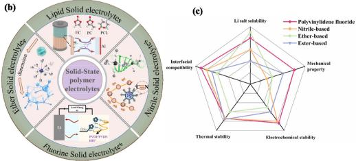
Fig. 1 Schematic illustration of a battery. (a) Li<sup>+</sup> transport in polymer electrolytes and growth of lithium dendrites, (b) typical polymer electrolytes, (c) Radar map of properties of different polymers.
