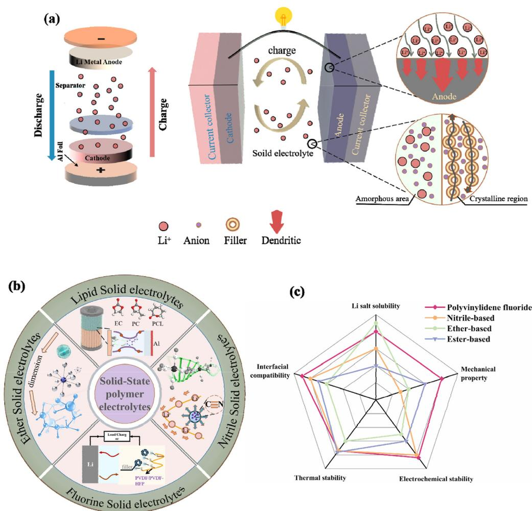
**Fig. 1** Schematic illustration of a battery. (a) Li<sup>+</sup> transport in polymer electrolytes and growth of lithium dendrites, (b) typical polymer electrolytes, (c) Radar map of properties of different polymers.
