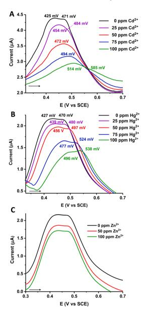
Fig. 5 Evolution of the SWV of the carbon paste working electrode prepared with ferrocenyl-functionalized material 2, recorded in a 0.1 M water solution of  $[NH_4][PF_6]$ , when increasing amounts of  $Cd^{2+}$  (A),  $Hg^{2+}$  (B) or  $Zn^{2+}$  (C) cations were added.
