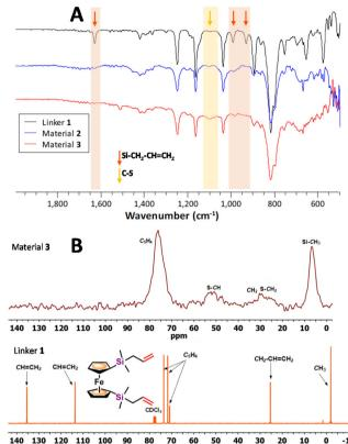
Fig. 1 (A) ATR-IR spectrum comparison of starting diallylsilyl-functionalized ferrocene 1 and materials 2 and 3. (B) SS  $^{13}$ C CP/MAS NMR spectrum of material 3 (up) and  $^{13}$ C NMR spectrum in CDCl<sub>3</sub> (300 MHz) of starting 1 (down).
