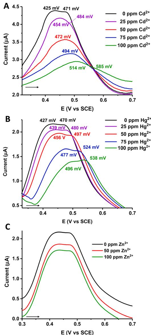
Fig. 5 Evolution of the SWV of the carbon paste working electrode prepared with ferrocenyl-functionalized material 2, recorded in a 0.1 M water solution of [NH<sub>4</sub>][PF<sub>6</sub>], when increasing amounts of Cd<sup>2+</sup> (A), Hg<sup>2+</sup> (B) or Zn<sup>2+</sup> (C) cations were added.
