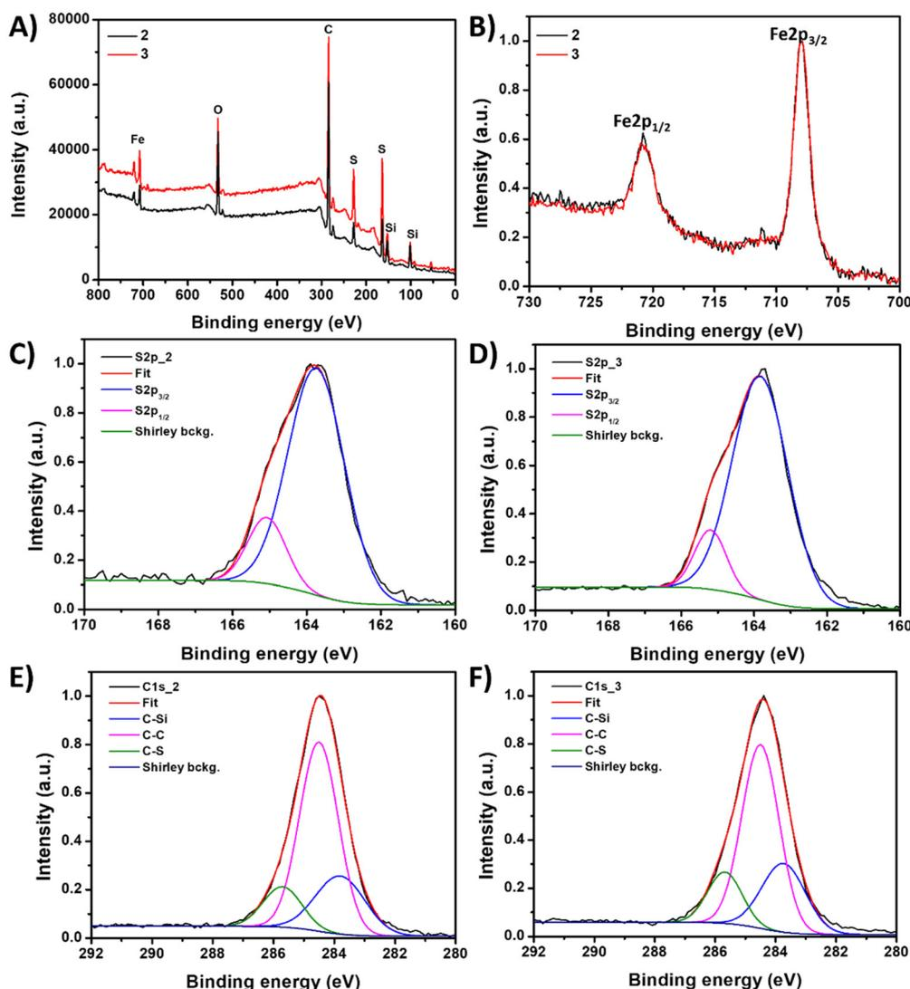
Fig. 2 (A) XPS spectra of material **2** (black line) and **3** (red line) samples. (B) XPS spectra of both samples in the Fe 2p region. (C and D) Fit spectra of the S 2p region for materials **2** and **3**, respectively. (E and F) Fit spectra of the C 1s region for materials **2** and **3**, respectively.
