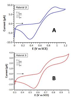
Fig. 4 Cyclic voltammograms (first cycle shown of the 10 cycles measured in each case) of materials 2 (A) and 3 (B) measured with a carbon paste working electrode, in a  $10^{-1}$  M CH<sub>3</sub>CN solution of  $[n-Bu_4N][PF_6]$ , at 50 mV s<sup>-1</sup>.
