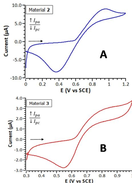
**Fig. 4** Cyclic voltammograms (first cycle shown of the 10 cycles measured in each case) of materials **2** (A) and **3** (B) measured with a carbon paste working electrode, in a  $10^{-1}$  M  $\text{CH}_3\text{CN}$  solution of  $[\text{n-Bu}_4\text{N}][\text{PF}_6]$ , at  $50 \text{ mV s}^{-1}$ .
