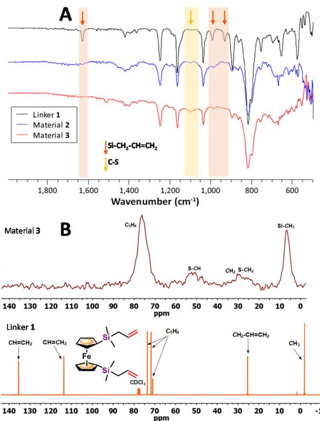
**Fig. 1** (A) ATR-IR spectrum comparison of starting diallylsilyl-functionalized ferrocene **1** and materials **2** and **3**. (B) SS  $^{13}\text{C}$  CP/MAS NMR spectrum of material **3** (up) and  $^{13}\text{C}$  NMR spectrum in  $\text{CDCl}_3$  (300 MHz) of starting **1** (down).
