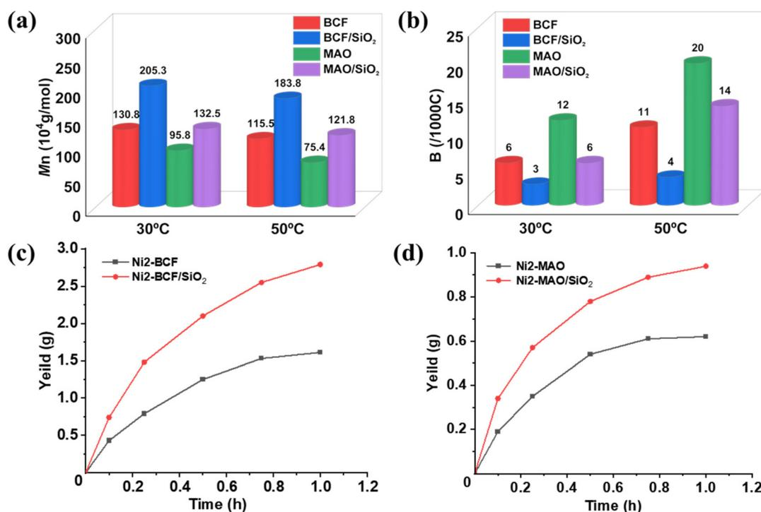
**Fig. 3** Comparisons of the homogeneous and heterogeneous ethylene polymerization systems using  $\text{Ni2}$ : (a) molecular weight comparisons of generated polyethylene at 30  $^\circ\text{C}$  and 50  $^\circ\text{C}$ ; (b) branching degree comparisons of generated polyethylene at 30  $^\circ\text{C}$  and 50  $^\circ\text{C}$ ; (c and d) time-dependent studies (polymer yields vs. polymerization time) at 80  $^\circ\text{C}$ .
