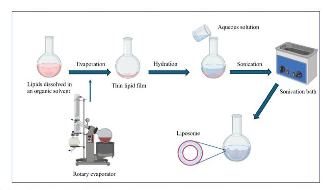
Fig. 5 Thin-film hydration method of liposomes preparation.
