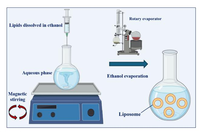
Fig. 6 Solvent injection method of liposomes preparation using ethanol.
