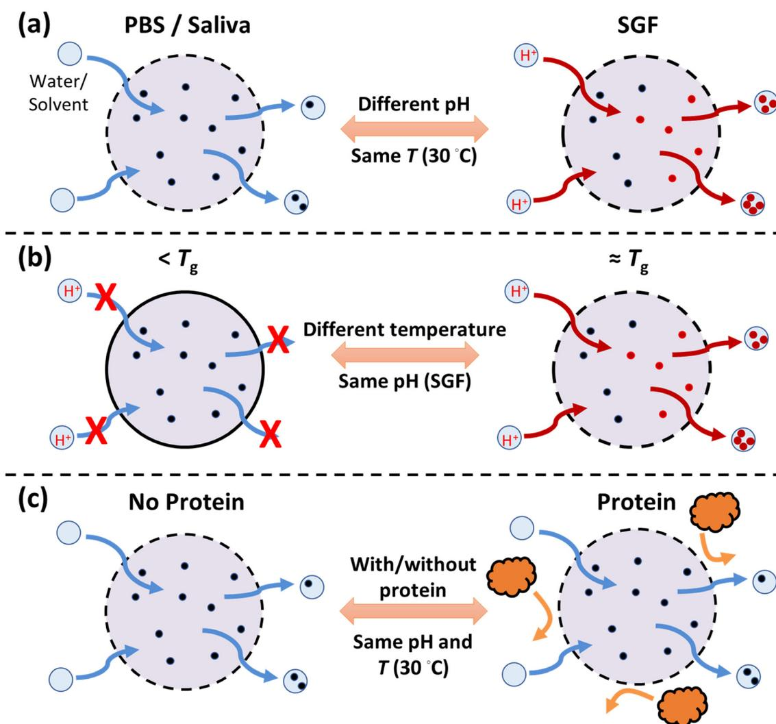
**Fig. 6** Schematic of drug release mechanisms in media at different pH (a), at temperatures below or near the glass transition temperature,  $T_g$  (b), with or without proteins (c). The roles of solvent intrusion and enrofloxacin charge state in SGF are emphasized, along with the lack of drug-protein interactions.
