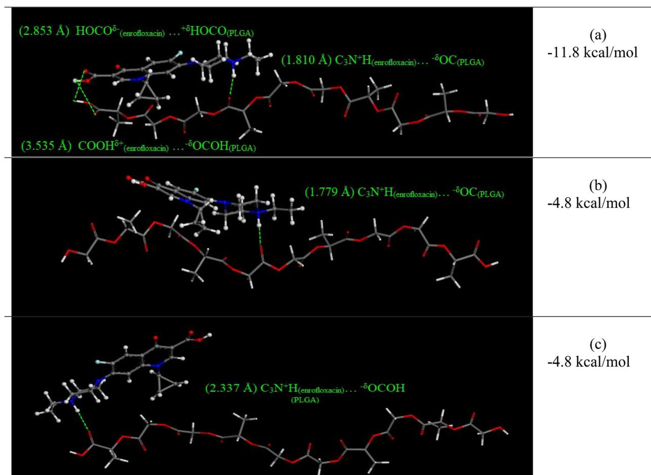
**Fig. 5** The optimized geometries for the enrofloxacin-PLGA interactions and their corresponding binding energies for cationic enrofloxacin interacting with protonated (neutral) carboxylated PLGA in three configurations (a, b, and c). Density functional theory (DFT) modeling of the zwitterionic and anionic enrofloxacin interacting with deprotonated PLGA are presented in our prior publication.<sup>16</sup>
