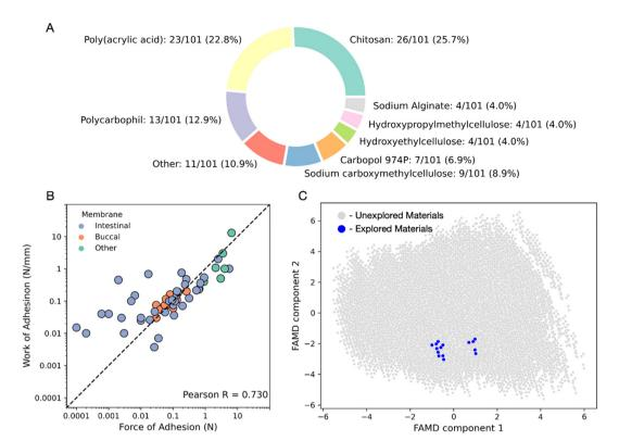
Fig. 3 Properties of published mucoadhesive polymers. (A) Proportions of base polymer units used in 101 published polymers assessed for mucoadhesion. (B) Correlation between force of adhesion (N), and work of adhesion (N mm<sup>-1</sup>) for 101 published polymers. (C) Total landscape of unexplored (grey) and explored (blue) mucoadhesive materials using all possible combinations of published base polymer units and parameters. FAMD – Factor Analysis of Mixed Data.
