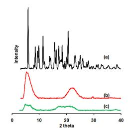
**Fig. 4** Powder X-ray diffractograms of (a) EFE, (b) mesoporous silica and (c) EFESD.
