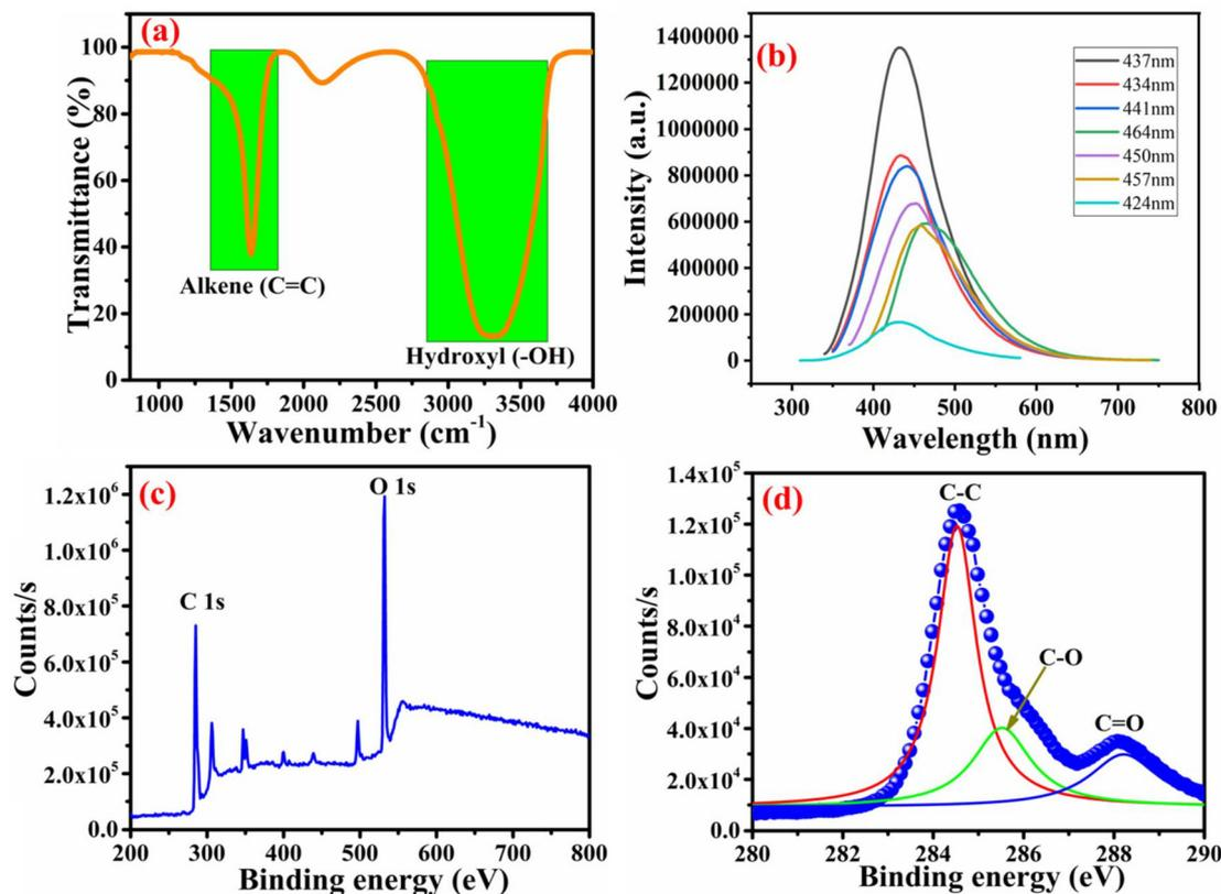
**Fig. 3** (a) FTIR of CQDs confirms the functional groups and purity of the synthesized carbon quantum dots. (b) PL spectrum shows that the carbon quantum dots are uniformly distributed. (c) XPS survey spectrum of CQDs and (d) XPS reveals no contaminants and confirms the purity of the PCQDs.
