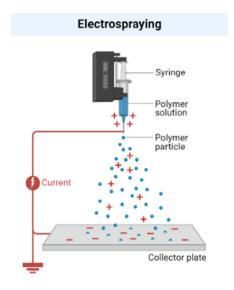
Fig. 7 A method of electrospinning and electrospraying by which DMAP, AAP, and HPβCD can be deposited to formulate patches with wound healing properties.  $^{174}$  Declaration: The figure was adapted from the open-source platform of "Biorender" tools (or templates). Reuse of its tools or templates has been allowed by "Biorender" (therefore, copyright is not applicable) with relevant previous citations (if any) being incorporated.  $^{171}$
