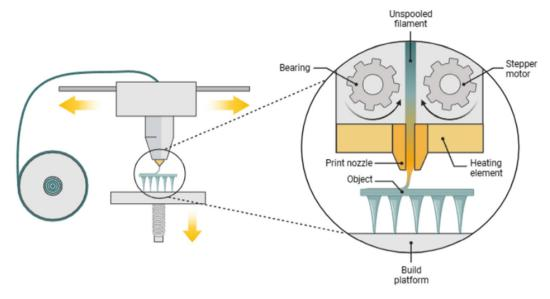
Fig. 5 Basic designs of a transdermal patch with 3D printing technology and using a fused deposition model. Declaration: The figure was adapted from the open-source platform of "Biorender" tools (or templates). Reuse of its tools or templates has been allowed by "Biorender" (therefore, copyright is not applicable) with relevant previous citations (if any) being incorporated.<sup>147</sup>
