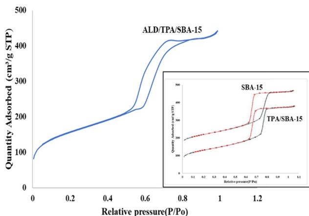
Fig. 6 Nitrogen ( $N_2$ ) adsorption-desorption isotherm of ALD/TPA/SBA-15.
