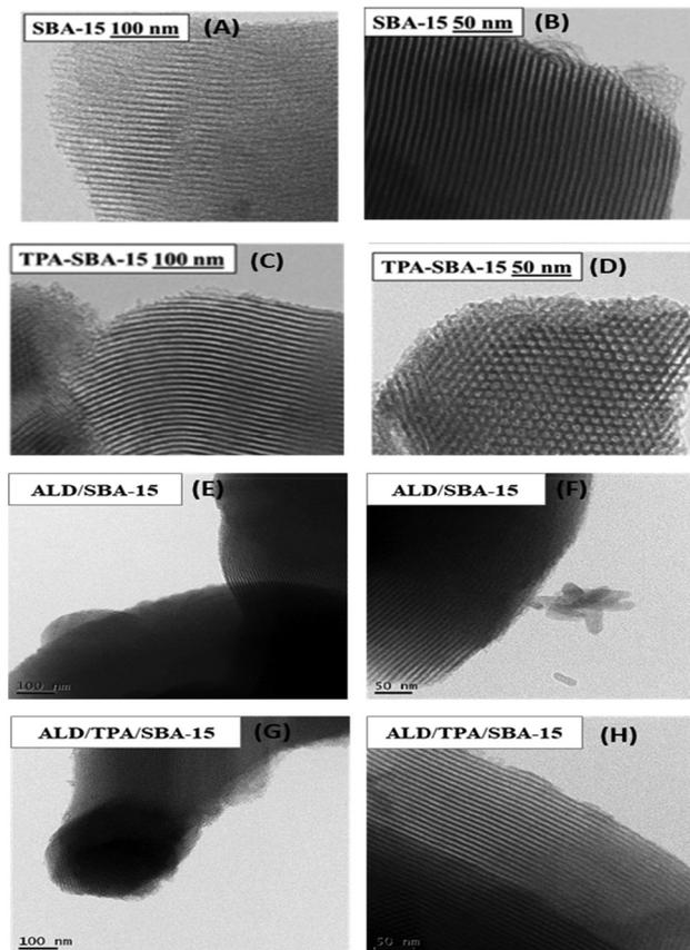
Fig. 7 HRTEM micrograph of (A and B) SBA-15, (C and D) TPA-SBA-15, (E and F) ALD/SBA-15, (G and H) ALD/TPA/SBA-15.
