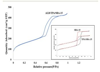
Fig. 6 Nitrogen (N<sub>2</sub>) adsorption-desorption isotherm of ALD/TPA/ SBA-15.
