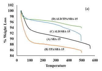
Fig. 2 (a) TGA curves of (A) SBA-15, (B) TPA-SBA-15, (C) ALD/SBA-15, (D) ALD/TPA/SBA-15.
