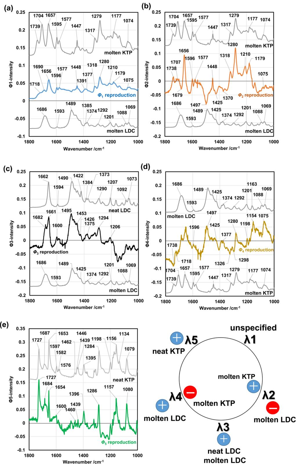
Fig. 6 Reproduction basis vector ( $\phi$ ) showing the spectral change of each component;  $\Phi_1$  (a),  $\Phi_2$  (b),  $\Phi_3$  (c),  $\Phi_4$  (d), and  $\Phi_5$  (e). Summarized scheme of the obtained components by the SVD analysis (f).
