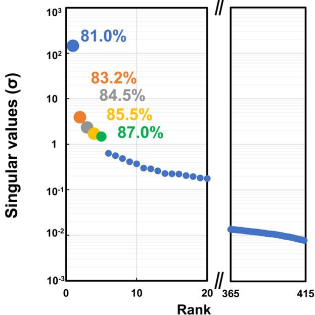
Fig. 5 Singular values ( $\sigma$ ) and cumulative contribution ratio obtained by SVD analysis of IR spectra.
