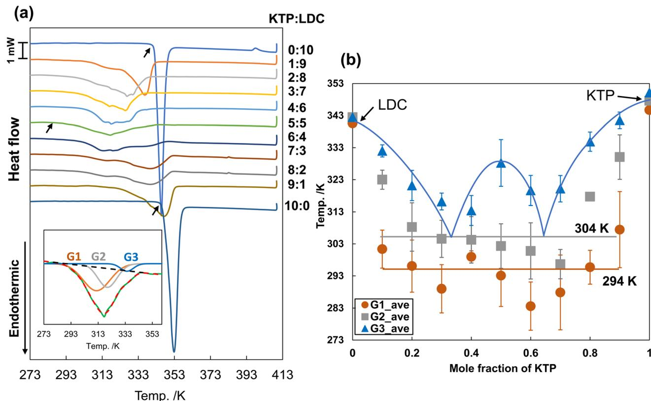
Fig. 4 (a) DSC thermograms of KTP/LDC mixtures with various ratios at a heating rate of  $5.0 \text{ K min}^{-1}$  ( $n = 3$ ). Black arrows show the melting points of neat LDC, neat KTP, and 5 : 5 mixture. (b) Binary solid–liquid phase diagram of melting points of KTP/LDC system at a heating rate of  $5.0 \text{ K min}^{-1}$ . Each plot is the average of values obtained from three experiments.
