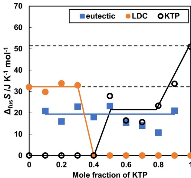
Fig. 3 Entropy of fusion in KTP and LDC upon heating of the KTP/LDC mixtures.  $\Delta_{\text{fus}}S^{\text{LDC}}$ ,  $\Delta_{\text{fus}}S^{\text{KTP}}$ , and  $\Delta_{\text{fus}}S^{\text{eutec}}$  are shown by orange closed circles, black open circles, and blue closed squares.
