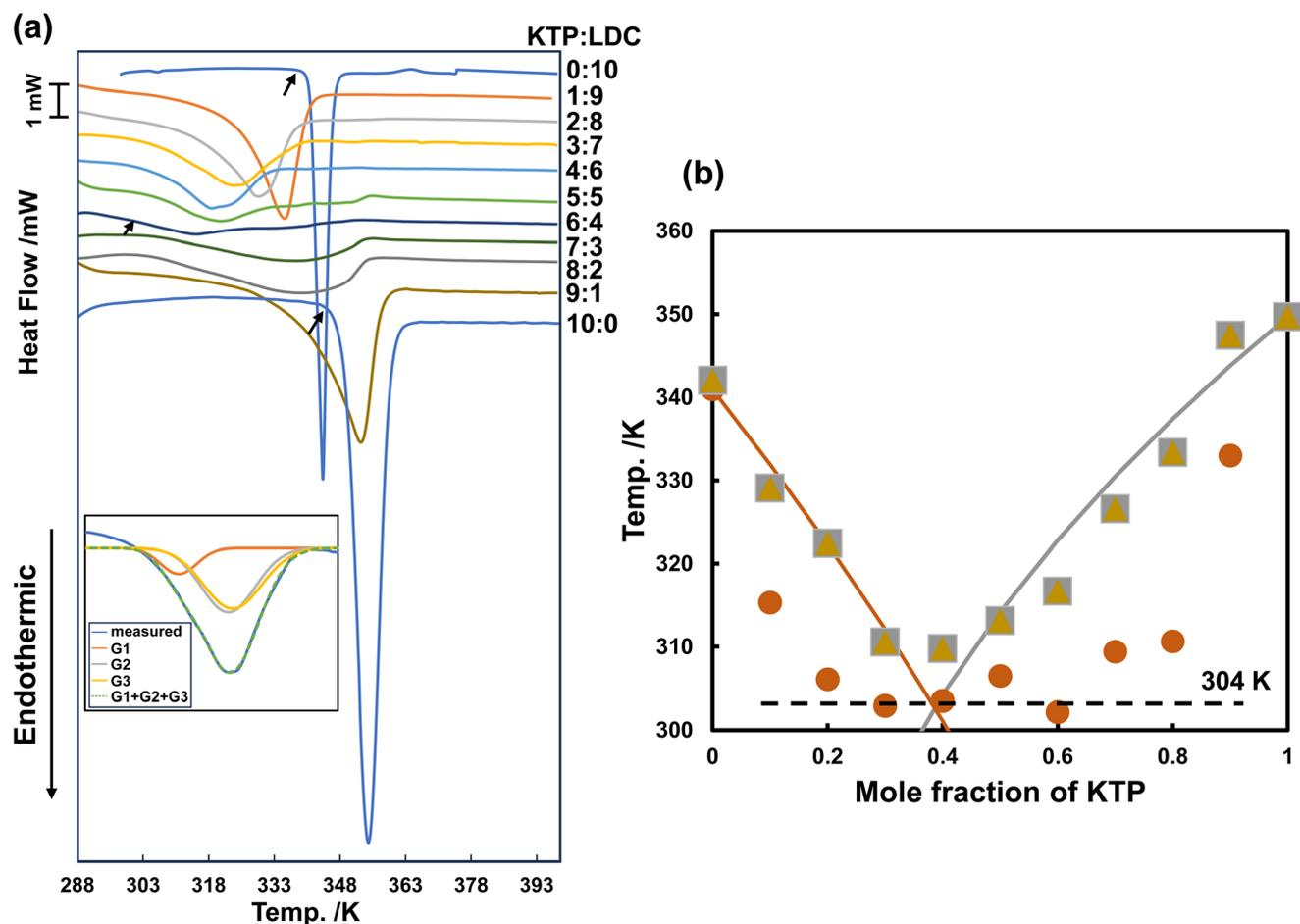
Fig. 2 (a) DSC thermograms of KTP/LDC mixtures with various ratios at a heating rate of  $10.0 \text{ K min}^{-1}$  ( $n = 1$ ). Black arrows show the melting points of neat LDC, neat KTP, and 6 : 4 mixtures. (b) Binary solid–liquid phase diagram of melting points of KTP/LDC system at a heating rate of  $10.0 \text{ K min}^{-1}$ . The phase transition temperatures were calculated from the obtained Gaussians, orange circles (G1), yellow squares (G2), and gray triangles (G3), respectively.
