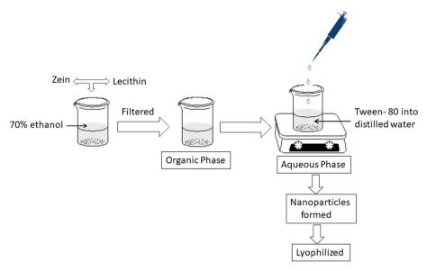
Fig. 1 Synthesis of zein encapsulated nanoparticles using the anti-solvent precipitation methodology. 17
