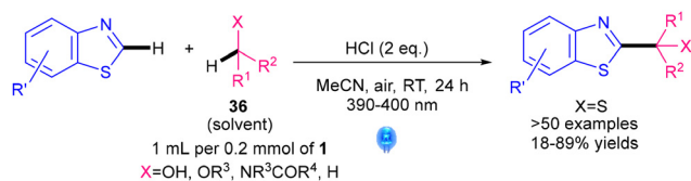
Scheme 27 "Self-catalysed" alkylation of benzothiazoles. 53
