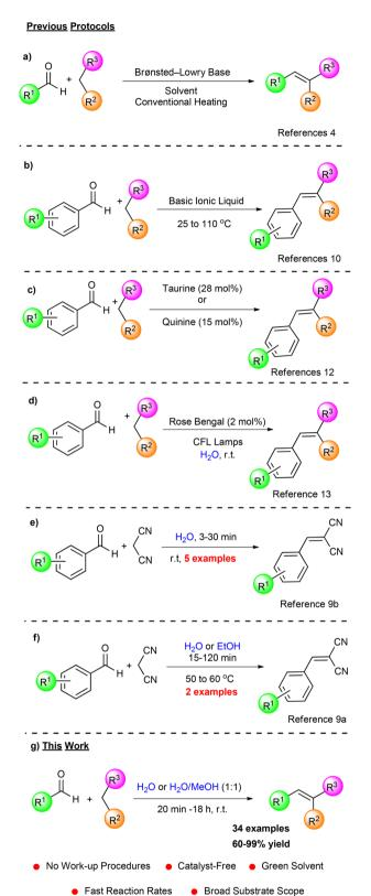
Scheme 1 Known synthetic pathways for the Knoevenagel condensation of aldehydes with active methylene compounds (a-f) and this work (g).
