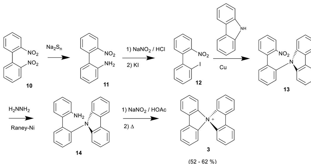
**Scheme 4** Hellwinkel's synthesis of spirodiphenylcarbazolium **3**.
