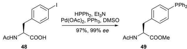
**Scheme 10** Palladium-catalysed synthesis of phosphine-containing aromatic amino acids – Kraatz and co-workers.<sup>25</sup>
