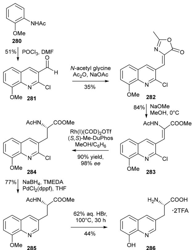
**Scheme 56** Asymmetric synthesis of 8HQ-3Ala via Rh-catalysed hydrogenation of a dehydroamino acid precursor – Banwell and co-workers.<sup>186</sup>
