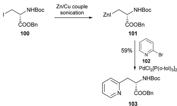
**Scheme 22** Synthesis of  $\beta$ -(2-pyridyl)alanine *via* palladium-catalysed cross coupling of the organozinc reagent **100** with 2-bromopyridine **102** – Jackson and co-workers.<sup>72</sup>
