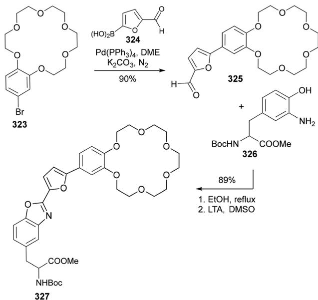
Scheme 64 Synthesis of a benzocrown ether amino acid featuring a furan spacer unit – Costa and co-workers.<sup>210</sup>
