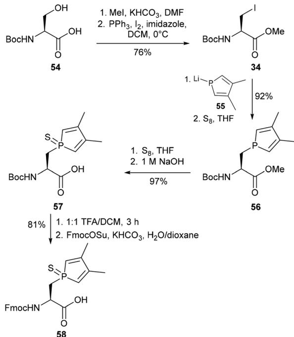
Scheme 12 Synthesis of a phosphole-containing amino acid 58 – Le Floch and co-workers.<sup>37</sup>
