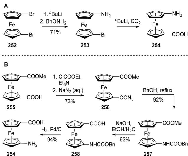
**Scheme 50** Synthesis of 1'-aminoferrocene-1-carboxylic acid by (A) lithiation and carboxylation, and (B) Curtius rearrangement and hydrogenolysis.<sup>175,176</sup>
