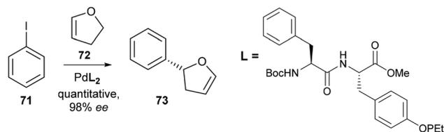
**Scheme 16** Asymmetric Heck reaction catalysed by a Pd(II) complex containing the dipeptide phosphinite ligand Boc-Phe-Tyr(OPEt<sub>2</sub>)OMe – Kraatz and co-workers.<sup>47</sup>
