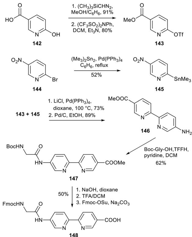
**Scheme 29** Synthesis of the  $\omega$ -amino acid XBp containing a bipyridyl group – Imperiali and co-workers.<sup>100</sup>
