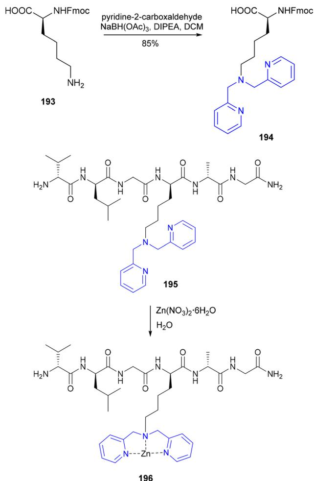
**Scheme 39** Synthesis of lysine derivative **194** containing a metal-binding dipicolylamine moiety (highlighted in blue) and its use in the preparation of the  $\text{Zn}^{2+}$ -binding peptide Val–Leu–Gly–**194**–Ala–Gly– $\text{NH}_2$  – König and co-workers.<sup>120</sup>
