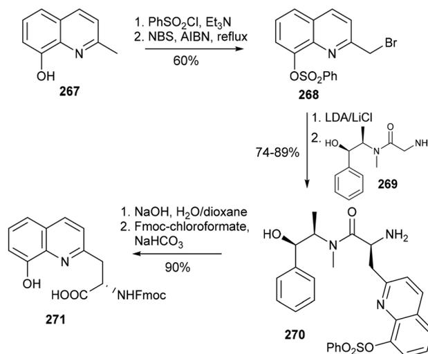
**Scheme 53** Asymmetric synthesis of an amino acid containing the 8-hydroxyquinoline scaffold – Imperiali and co-workers.<sup>182</sup>
