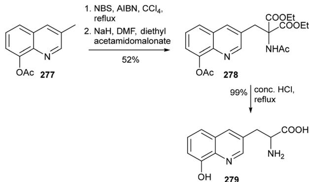
**Scheme 55** Racemic synthesis of a 3-substituted amino acid containing the 8-hydroxyquinoline scaffold – Schultz and co-workers.<sup>185</sup>
