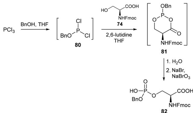
**Scheme 18** One-pot process for the synthesis of phosphoserine derivatives – Bakale and co-workers.<sup>54</sup>
