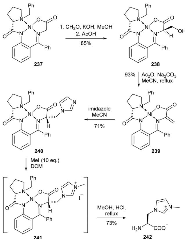
**Scheme 47** Synthesis of an imidazolyl amino acid using a chiral masked glycine Ni(II) complex – Belokon and co-workers.<sup>142</sup>
