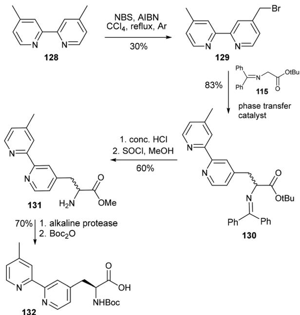
**Scheme 27** Synthesis of an *N*-Boc protected 4-methyl-2,2'-bipyridyl amino acid – Bowler and co-workers.<sup>97</sup>
