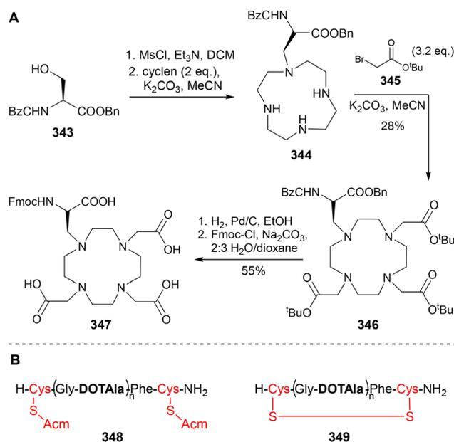
**Scheme 67** (A) Synthesis of DOTAla X and (B) peptide sequences assembled by Fmoc SPPS incorporating up to 3 repeating DOTAla residues – Caravan and co-workers.<sup>215</sup>
