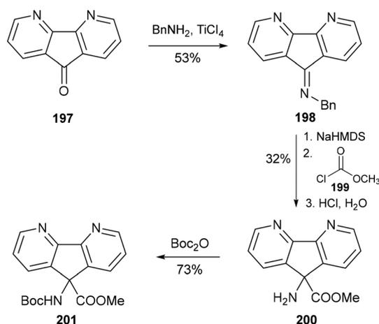
**Scheme 40** Synthesis of an  $\alpha$ -disubstituted amino acid functionalised with a rigid 2,2'-bipyridine ligand – Toniolo and co-workers.<sup>124</sup>
