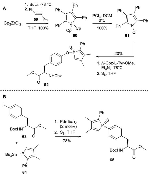
Scheme 13 Functionalisation of aromatic amino acids with a phosphole moiety *via* (A) nucleophilic substitution and (B) Stille cross-coupling – Le Floch and co-workers.<sup>38</sup>
