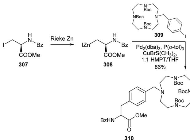
**Scheme 60** Synthesis of a phenylalanine derivative containing a cyclen moiety in the sidechain by Negishi coupling – König and co-workers.<sup>201</sup>
