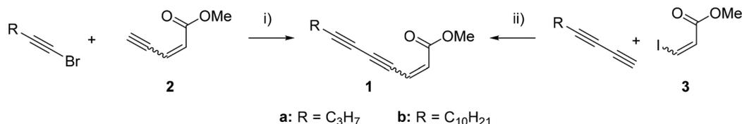
**Scheme 3** Synthesis of *Lachnophyllum* methyl esters *Z*-1a and *E*-1a and their analogs *Z*-1b and *E*-1b. Reagents and conditions: (i) Cadiot-Chodkiewicz coupling: CuCl, NH<sub>2</sub>OH·HCl, *n*BuNH<sub>2</sub>, THF, 0 °C to rt; (ii) Sonogashira coupling: PdCl<sub>2</sub>(PPh<sub>3</sub>)<sub>2</sub>, CuI, Et<sub>3</sub>N, THF, 40 °C overnight.
