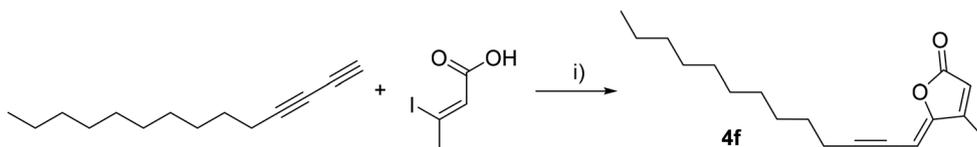
**Scheme 9** Synthesis of (4Z)-*Lachnophyllum* lactone analog **4f**. Reagents and conditions: (i) PdCl<sub>2</sub>(PPh<sub>3</sub>)<sub>2</sub>, CuI, Et<sub>3</sub>N, CH<sub>3</sub>CN, 40 °C overnight, 35%.
