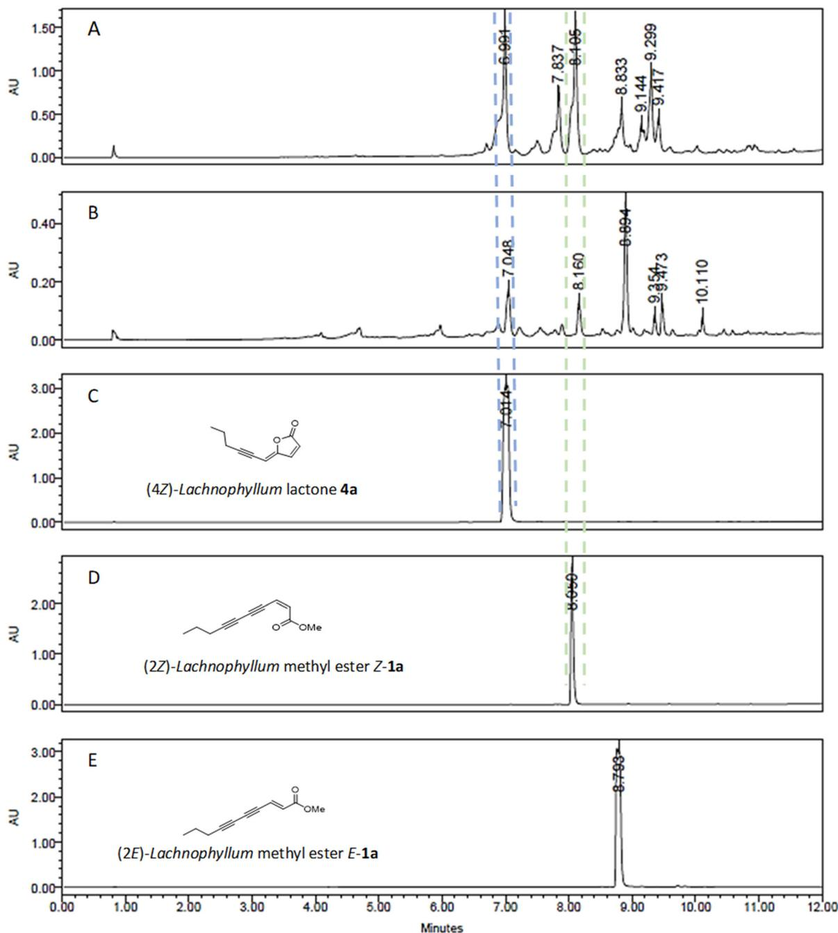
**Fig. 2** Analytical chromatograms obtained using an Acquity Premier BEH C18 1.7  $\mu\text{m}$  (2.1  $\times$  100) mm column,  $\text{H}_2\text{O}/\text{CH}_3\text{CN}$ , 0.1%  $\text{HCOOH}$  (95 : 5 to 0 : 100, 0.3  $\text{mL min}^{-1}$ , 40  $^\circ\text{C}$ , UV detection at 254 nm). (A) Hexanoic extract obtained according to Adande *et al.*;<sup>7</sup> (B) heptanoic extract obtained by ASE; (C) compound **4a**; (D) compound **Z-1a**; (E) compound **E-1a**.
