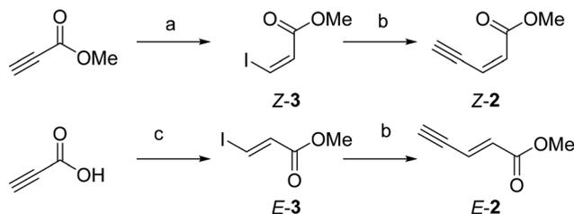
**Scheme 2** Synthesis of methyl 3-iodoacrylates **Z-3** and **E-3** and methyl pent-2-en-4-ynoates **Z-2** and **E-2**. Reagents and conditions: (a) NaI, AcOH, 70 °C, 84%; (b) (i) TMS-C≡CH, PdCl<sub>2</sub>(PPh<sub>3</sub>)<sub>2</sub>, CuI, Et<sub>3</sub>N, THF, 0 °C to rt; (ii) TBAF, THF, 0 °C to rt, 68% over two steps for **Z-2**, 76% over two steps for **E-2**; (c) (i) HI, H<sub>2</sub>O, reflux, (ii) H<sub>2</sub>SO<sub>4</sub>, MeOH, reflux, 74% over two steps.
