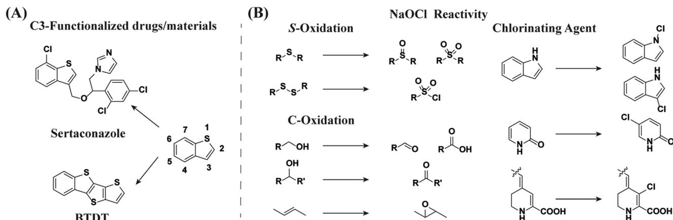
**Fig. 1** (A) The numbering system of benzo[*b*]thiophene along with a drug displaying C3-functionalization, as well as a functional derivative that can be obtained from C3-functionalization of benzo[*b*]thiophene.<sup>39</sup> (B) Examples of the most common reactions of sodium hypochlorite pentahydrate as an oxidant or a chlorination agent, with references mentioned within the text.
