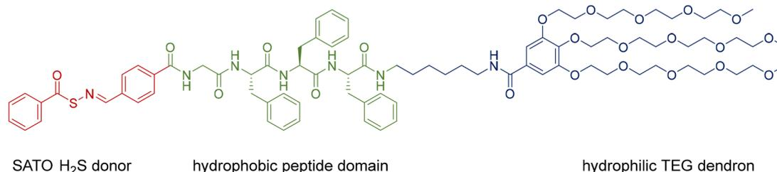
**Fig. 1** Chemical structure of the H<sub>2</sub>S-releasing amphiphilic SATO-GFFF-TEG dendron PHDC (referred to simply as the PHDC), including the SATO H<sub>2</sub>S donor (red); the hydrophobic peptide domain GFFF (green); and the hydrophilic TEG dendron segment (blue).
