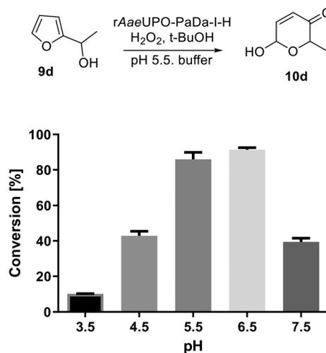
**Fig. 1** pH profile of the rAaeUPO-PaDa-I-H catalysed transformation of **9d** into **10d**. Reactions were performed in 150  $\mu$ L total volume, extracted with 2 × 200  $\mu$ L EtOAc and analysed by GC-FID on a HP-5MS column (30 m) at RT.<sup>33</sup> Citrate buffers were used between pH 3.50 and 5.50 (50 mM) and above this KPi buffers (50 mM) were employed. Error bars show  $\pm$ one standard deviation from the mean.
