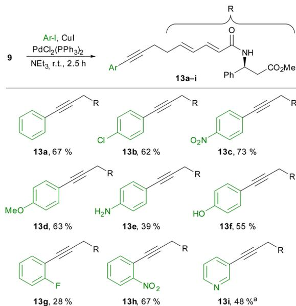
**Scheme 4** Sonogashira coupling of alkyne **9** with various aryl iodides. <sup>a</sup>The reaction was performed for 2 h at 60 °C.
