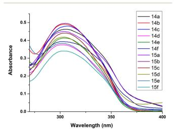
Fig. 2 UV/Vis absorption spectra for compounds 14a–f and 15a–f in DMSO at 2  $\times$  10<sup>-5</sup> M concentration.
