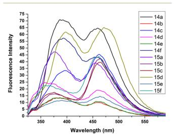
Fig. 3 Emission spectra for compounds 14a–f and 15a–f in DMSO at 2  $\times$  10<sup>-5</sup> M concentration (excitation at  $\lambda_{ex}$  = 300 nm).
