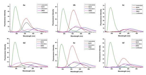
Fig. 5 Emission spectra for fluorophores 6a-f in acetonitrile, MeOH, chloroform, DMSO and 1,4-dioxane at  $2 \times 10^{-5}$  M concentration (excitation at  $\lambda_{\rm ex}$  = 250 nm).
