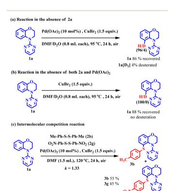
**Scheme 7** H/D exchange and kinetic experiment.
