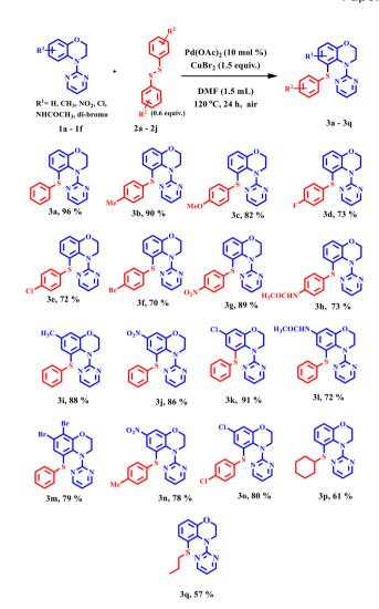
Scheme 1 Scope of sulfenylation of 4-(pyrimidin-2-yl)-3,4-dihydro-2H-benzo[b][1,4]oxazines.
