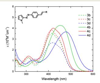
Fig. 3 Comparison of UV-Visible spectra of 3b-d (dotted line) and 4bd (continue line) acquired in MeOH.
