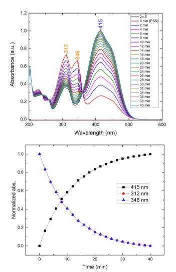
Fig. 6 (Top) UV-vis absorption spectra for 2a in the photo-stationary state after white led irradiation, and spectral evolution during the  $cis \rightarrow$ trans thermal return. (Dawn) Absorption changes during the  $cis \rightarrow trans$ thermal return at three different wavelengths.
