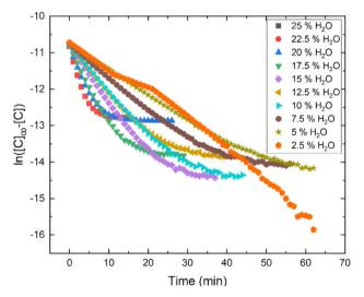
Fig. 10 (Top) UV-Vis spectra for 3b ( $2.9 \times 10^{-5}$  M, MeOH/H<sub>2</sub>O 80 : 20) after irradiation (PSS) and cis-trans return. The spectra were acquired every minute. (Dawn)  $ln([C]_{\infty} - [C])$  vs. time for 3b ( $2.9 \times 10^{-5}$  M) after white light irradiation in different ratios MeOH/H<sub>2</sub>O (the loss of linearity is observed).
