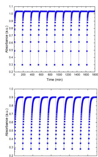
Fig. 7 Photoisomerization fatigue cycles for compounds 2a (top) and 4b (dawn). Samples were irradiated ten times for 2 minutes (5.0 mW).
