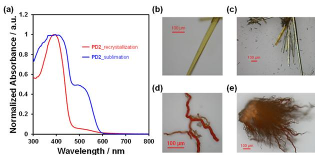
**Fig. 14** (a) Solid-state UV-vis diffuse reflectance-absorption spectra of the crystals of **PD2** and the solids of the sublimate obtained by heating the crystals of **PD2** at 133 °C under vacuum. Photographs of (b and c) the crystals and (d and e) the solids of the sublimate for **PD2**.
