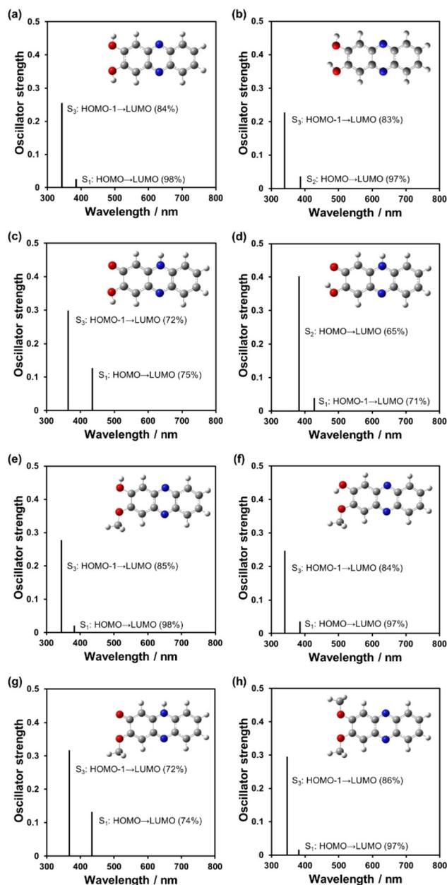
**Fig. 16** Calculated photoabsorption spectra of (a) *anti*-PD1-E, (b) *syn*-PD1-E, (c) *anti*-PD1-K, (d) *syn*-PD1-K, (e) *anti*-PD2-E, (f) *syn*-PD2-E, (g) PD2-K, and (h) PD3 derived from TDDFT calculations at the B3LYP/6-311G(d,p) level. For convenience of calculations, the methoxymethoxy groups of *anti*-PD2-E, *syn*-PD2-E, PD2-K, and PD3 were replaced with the methoxy groups.
