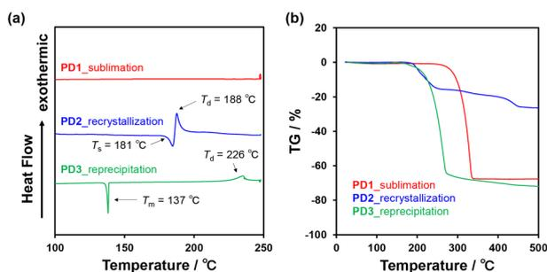
**Fig. 13** (a) DSC curves (heating process from 25 °C to 250 °C at a scan rate of 1 °C min<sup>-1</sup>) and (b) TG curves (heating process from 25 °C to 500 °C at a scan rate of 10 °C min<sup>-1</sup>) of **PD1-3**.
