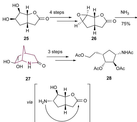
**Scheme 5** Synthesis of bicyclic system **27** by intramolecular cyclization.
