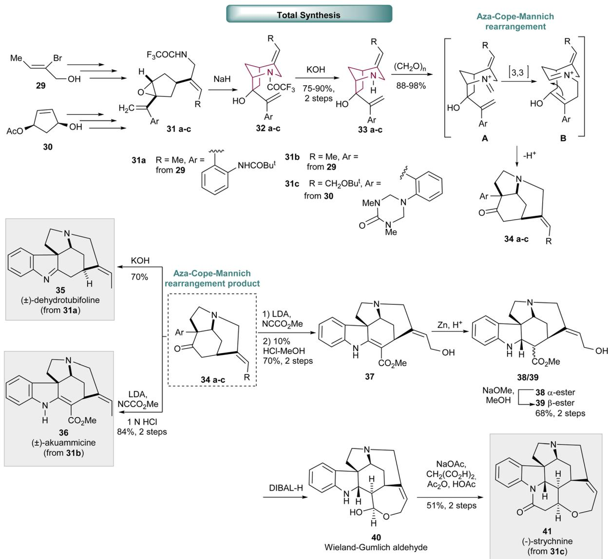
**Scheme 6** Synthesis of bicyclic system **32a–c** by intramolecular epoxide ring opening reaction. Aza-Cope-Mannich rearrangement of **33a–c** to **34a–c**, a key intermediate in the total synthesis of (±)-dehydrotubifoline **35**, (±)-akuammicine **36** and (-)-strychnine **41**.
