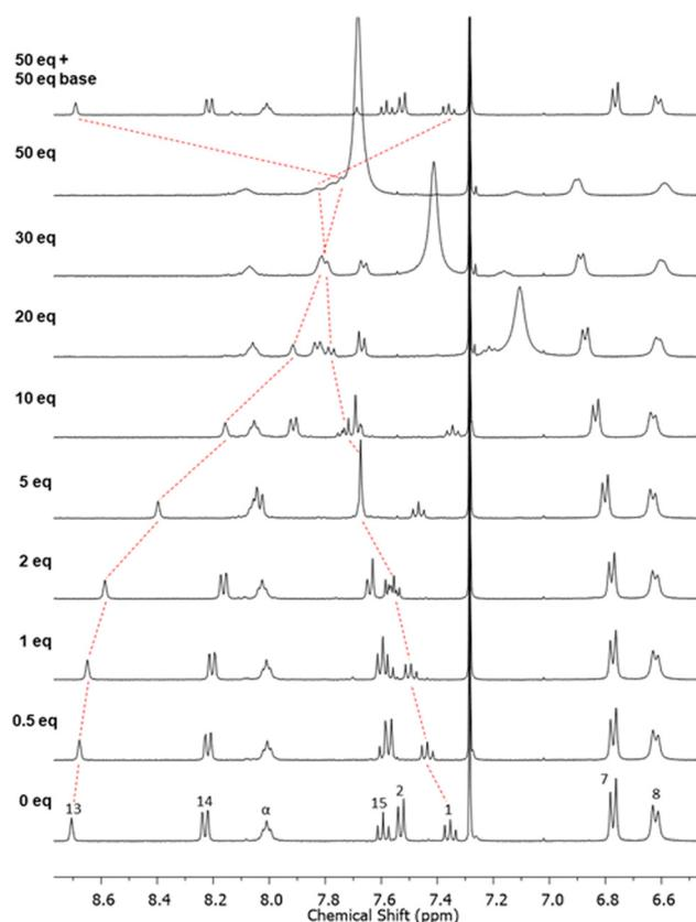
Fig. 3 Partial  $^1\text{H}$  NMR spectra and highlighted chemical shifts of diagnostic proton resonances of PNO [2]catenane 4 with set equivalent additions of TFA followed by reversal with the addition of  $d_5$ -pyridine ( $\text{CDCl}_3$ , 400 MHz, 298 K). NB: The large peak that appears in spectra for 20, 30 and 50 eq. of TFA is protic O-H.
