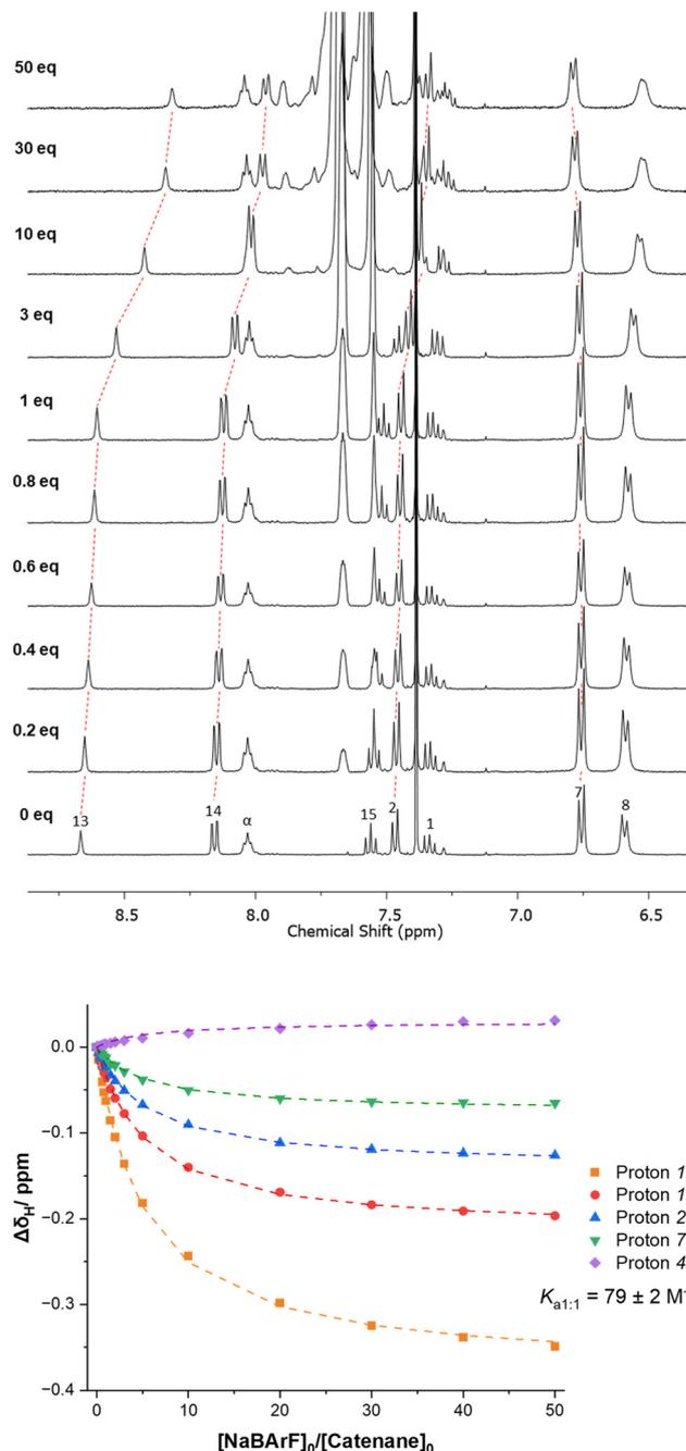
**Fig. 5** Partial  $^1\text{H}$  NMR spectra and highlighted chemical shifts of diagnostic proton resonances of PNO [2]catenane **4** with set equivalent additions of  $\text{NaBARF}$  (4 : 1  $\text{CDCl}_3/\text{CD}_3\text{CN}$ , 400 MHz, 298 K) and globally fitted data (by BindFit) for a 1 : 1 binding isotherm using change in peak positions against a ratio of initial cation and catenane concentration.
