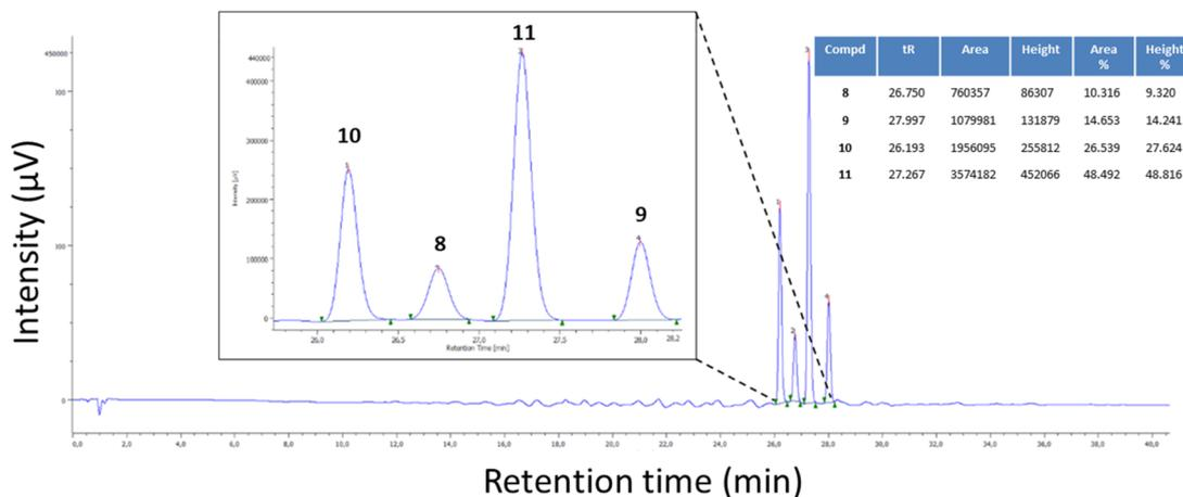
Fig. 3 Example of HPLC chromatogram of a mixture of compounds 8–11. HPLC method: RP-C18; flow: 0.4 mL min<sup>-1</sup>; 0.1% formic acid in H<sub>2</sub>O 100% to 0.1% formic acid in H<sub>2</sub>O 50% : CH<sub>3</sub>CN 50% in 40 min.
