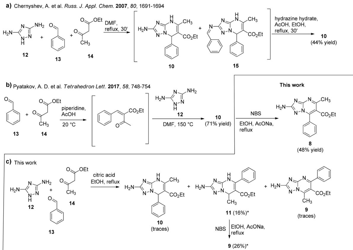
**Scheme 3** (a) and (b) Known procedures for the synthesis of **10**. (b) Oxidation of **10** to aromatic TZP **8** performed in this work. (c) Synthesis of **11** via the MCR of 3,5-diaminotriazole (**12**), benzaldehyde (**13**) and ethyl 3-oxobutanoate (**14**), and its oxidation to compound **9**, respectively. \*Isolated yield.
