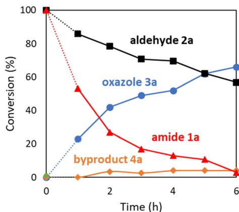
Fig. 2 Time course of the reaction for oxazole synthesis: amide **1a** (1 mmol), aldehyde **2a** (5 mmol), Pd(TFA)<sub>2</sub> (5 mol%), *n*-octane (4 mL), 150 °C, sealed tube, in air.
