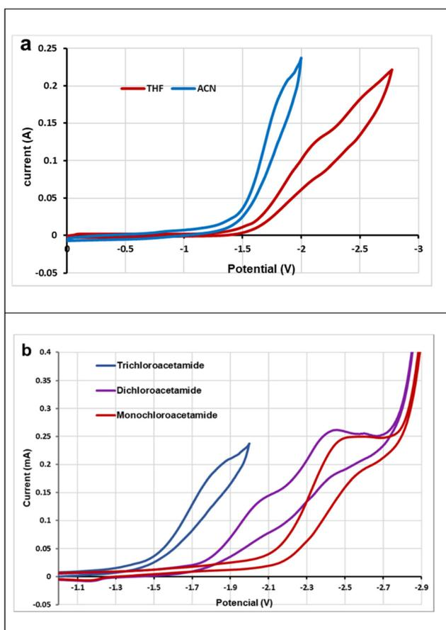
Fig. 5 (a) Cyclic voltammetric study of **1a** in THF and in acetonitrile. (b) Cyclic voltammetric study of trichloroacetamide **1a** and its analogues  $\alpha,\alpha$ -dichloro and  $\alpha$ -chloro acetamides in acetonitrile.
