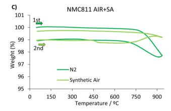
Fig. 6  $\,$  TGA results of (A) NMC811 AIR, (B) NMC811 SA, and (C) NMC811 AIR + SA.
