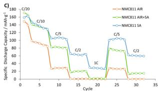
Fig. 8 (A)  $dQ_m/dV$  plots of the second formation C/20 cycle, (B) cycle stability at C/10, and (C) C-rate capability from C/20 to 5C of NMC811 calcined in air, in synthetic air (SA), and in air and synthetic air (AIR + SA).
