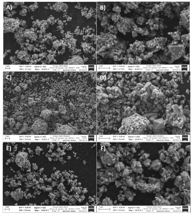
Fig. 2 SEM images at x10 000 and x25 000 magnifications of the NMC811 calcined in (A and B) air, (C and D) synthetic air, and (E and F) air and annealed in synthetic air.
