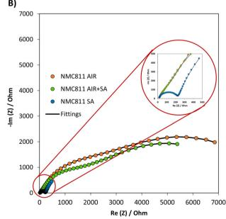
Nyquist plots for the NCM811 calcined in air (AIR), in synthetic air (SA), and in air and annealed in synthetic air (AIR + SA), (A) before and (B) after 50 cycles at C/10. The impedance was measured at a fully discharged electrode state.
