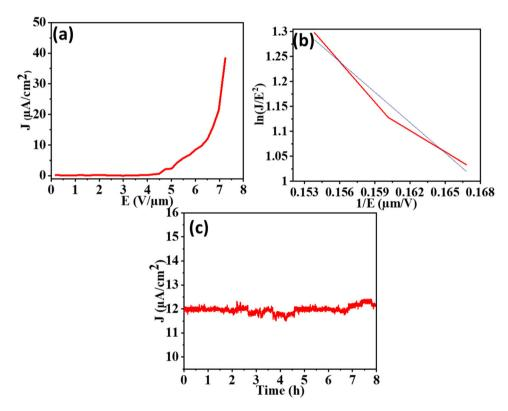
Fig. 8 (a) J-E plot, (b) F-N plot and (c) temporal stability of Bi<sub>2</sub>S<sub>3</sub>.
