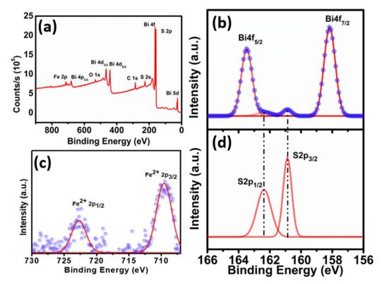
Fig. 6 (a) XPS survey spectrum of FeS-Bi<sub>2</sub>S<sub>3</sub> and high-resolution spectra of (b) Bi 4f, (c) Fe 2p and (d) S 2p.
