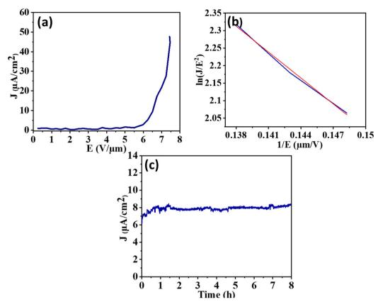
Fig. 9 (a) J-E plot. (b) F-N plot and (c) temporal stability of FeS-Bi<sub>2</sub>S<sub>3</sub>.
