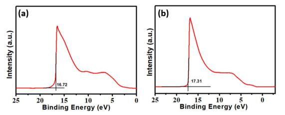
Fig. 7 UPS spectra of (a) Bi<sub>2</sub>S<sub>3</sub> and (b) FeS-Bi<sub>2</sub>S<sub>3</sub>.
