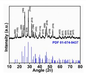
Fig. 1 PXRD pattern of Bi<sub>2</sub>S<sub>3</sub> nanorods.
