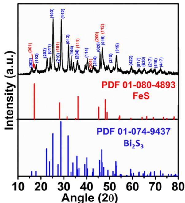
Fig. 3 PXRD pattern of FeS- $\text{Bi}_2\text{S}_3$  nanorods.
