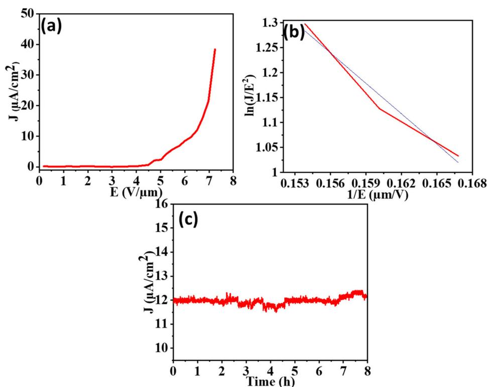
Fig. 8 (a)  $J$ - $E$  plot, (b)  $F$ - $N$  plot and (c) temporal stability of  $\text{Bi}_2\text{S}_3$ .
