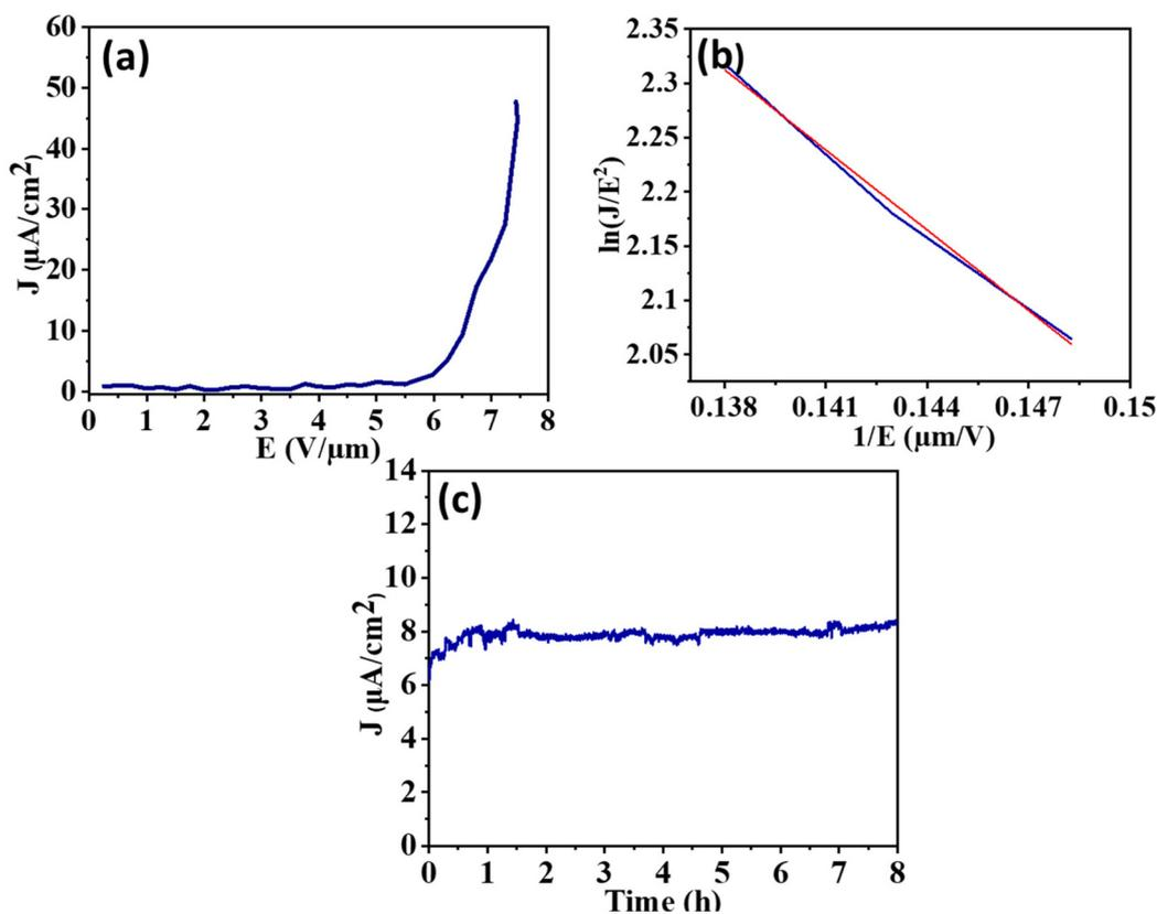
Fig. 9 (a)  $J$ - $E$  plot, (b)  $F$ - $N$  plot and (c) temporal stability of FeS-Bi<sub>2</sub>S<sub>3</sub>.
