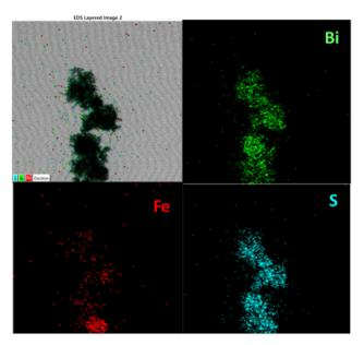
Fig. 5 TEM overlay image and elemental mapping of S, Bi and Fe in FeS-Bi<sub>2</sub>S<sub>3</sub>.
