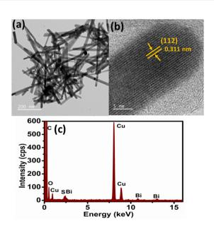
Fig. 2 (a) TEM micrograph, (b) HR-TEM image and (c) electron dispersive spectroscopy (EDS) spectrum of Bi<sub>2</sub>S<sub>3</sub> nanorods.
