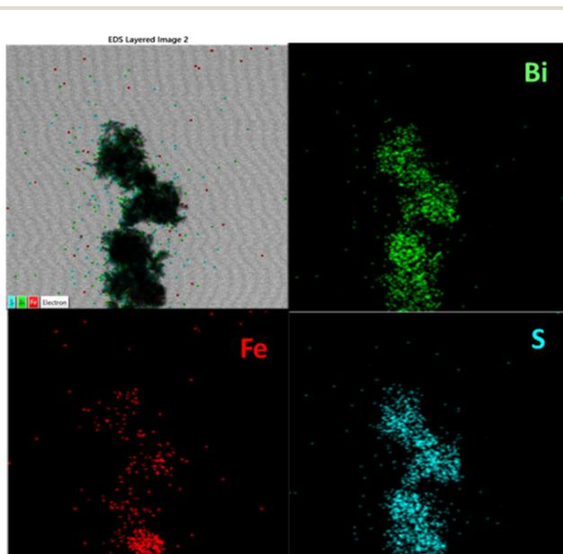
Fig. 5 TEM overlay image and elemental mapping of S, Bi and Fe in FeS- $\text{Bi}_2\text{S}_3$ .
