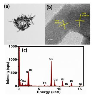
Fig. 4 (a) TEM micrograph, (b) HR-TEM image and (c) electron dispersive spectroscopy (EDS) spectrum of FeS-Bi<sub>2</sub>S<sub>3</sub> nanorods.
